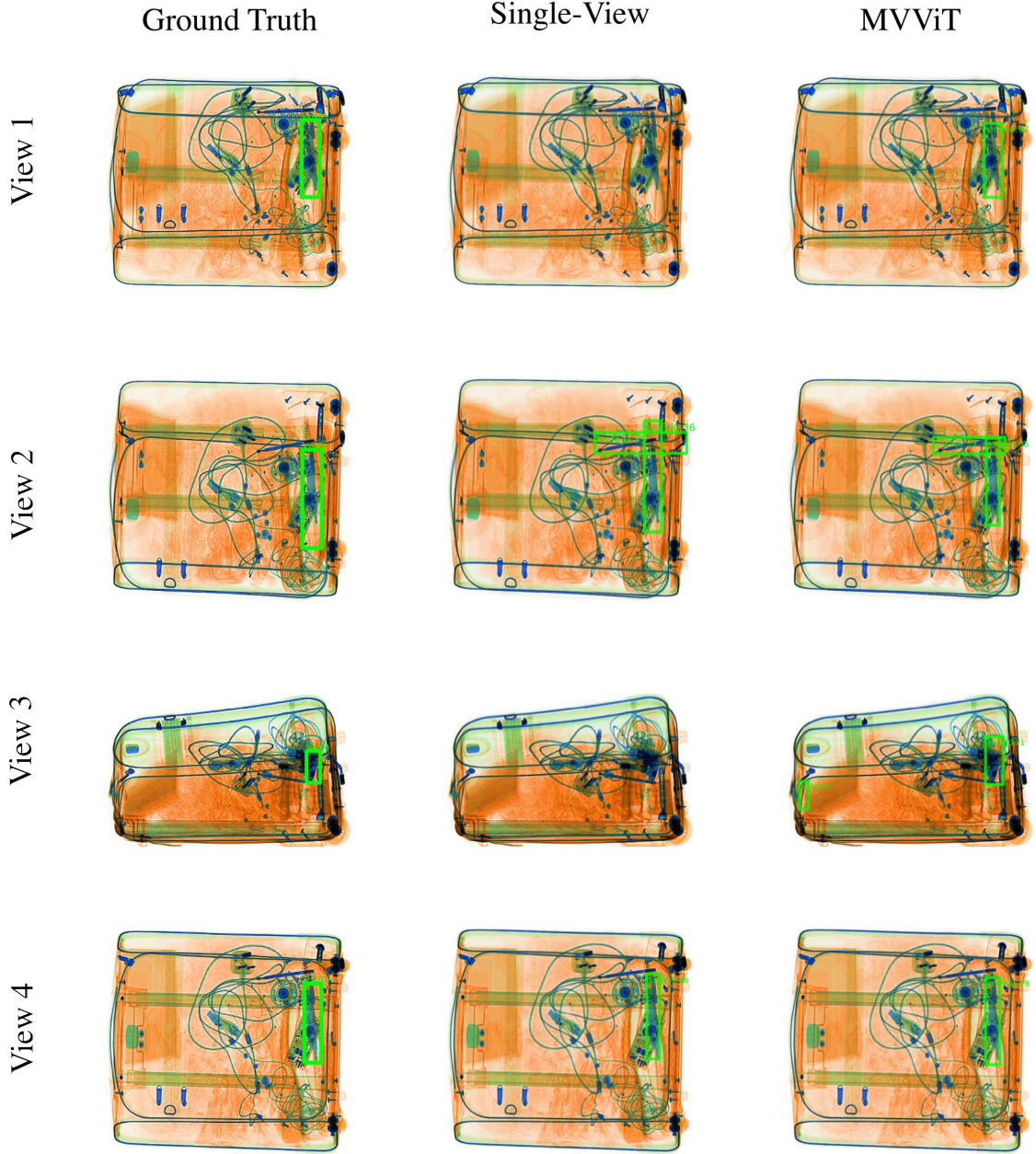
Figure 4.4: Single-view vs. Multi-view detection with MVViT on the X-ray-Quad dataset. Detector: Faster RCNN with a Swin Transformer backbone.
