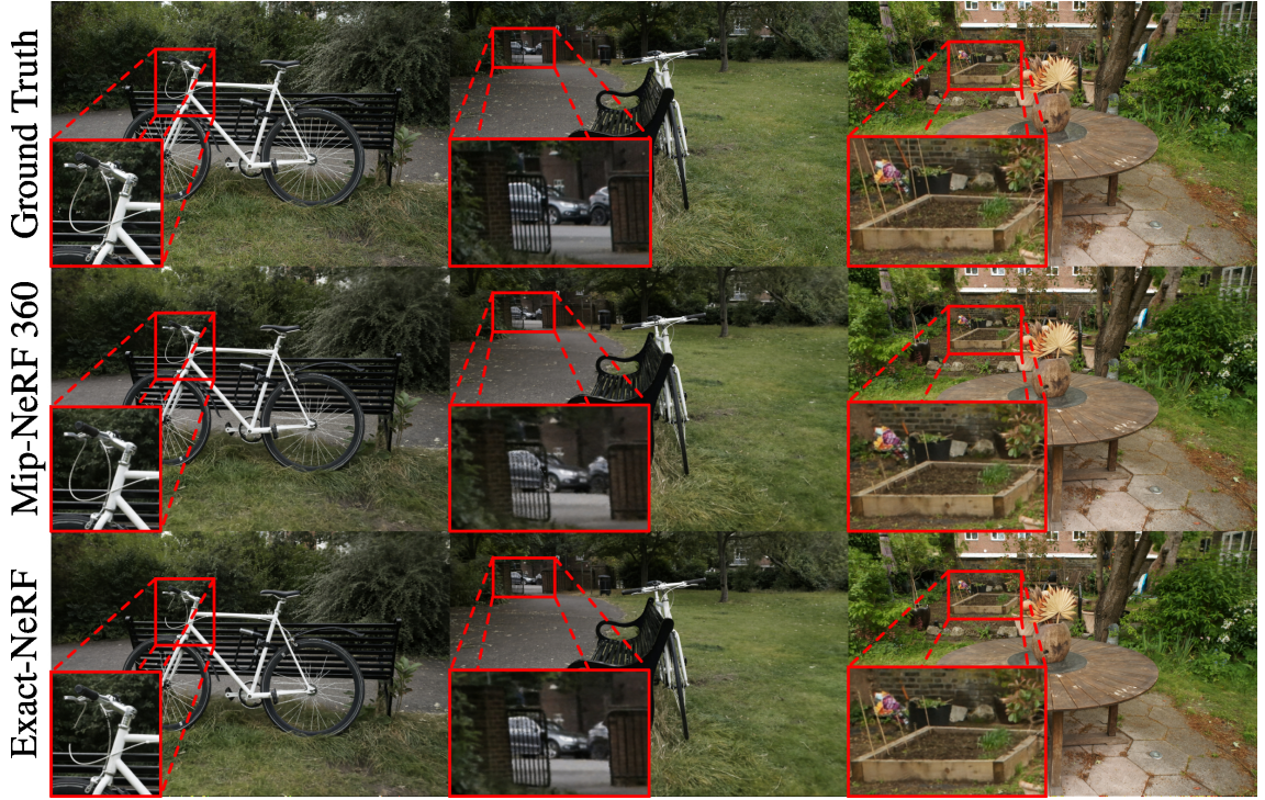
Figure 5.5: Qualitative comparison between mip-NeRF 360 and Exact-NeRF. Left-column : the proposed model, similar to mip-NeRF, struggles with tiny vessels. Middle-column : Exact-NeRF shows cleaner renderings. Right-column : Exact-NeRF has higher quality background reconstruction.
