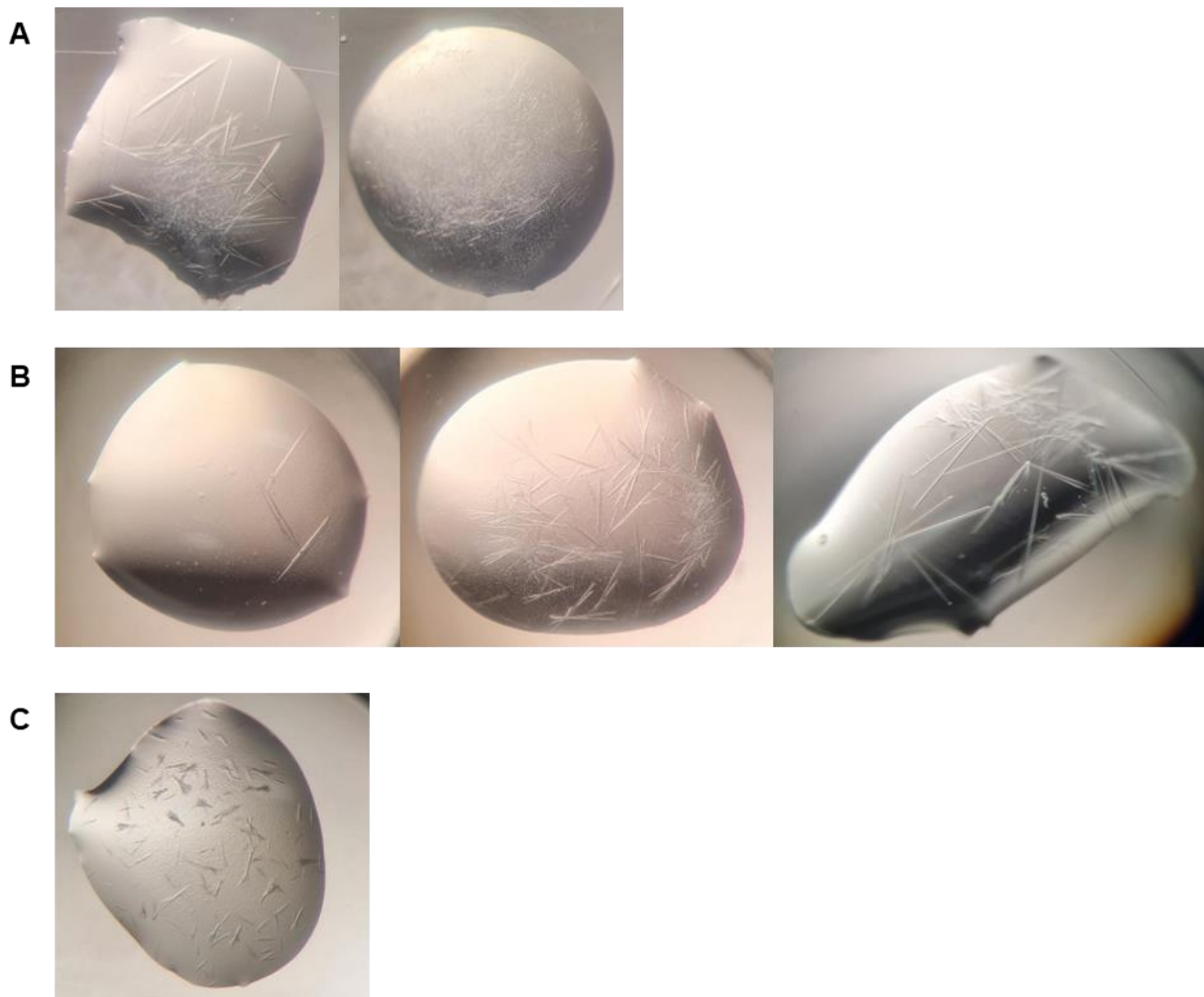
Figure 5.5 – PglX + SAM protein crystals. A selection of protein crystals from crystallisation screens using PglX co-incubated with Ocr. A; crystals from CSI optimisation round 1. B; crystals from CSI optimisation round 2. C; crystals representative of those produced by the commercially available screens, Morpheus I, Morpheus II and Morpheus Fusion (Molecular Dimensions).
