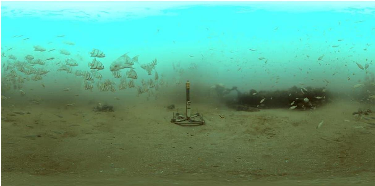
*Figure 1.1. Remote passive acoustic instrument deployed on the seabed (NOAA, 2018).*
