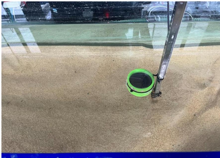
*Figure 2.6. Reversed hydrophone setup, with hydrophone pointing upwards towards water surface.*
