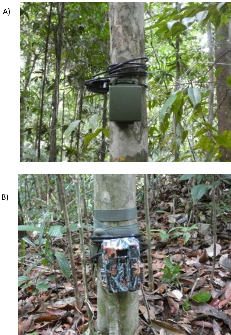
Figure 2.2 Photographs of the recording units used in the study namely: A) an Autonomous Recording Unit (SongMeters by Wildlife Acoustics) and B) a camera trap (Browning Recon Force Edge 4K). Recording pairs were deployed at 69 randomly generated recording sites for 30 days, with respective Python locks to prevent theft, at heights of approximately 2m and 50cm above ground level respectively to maximise efficient surveying capabilities.
