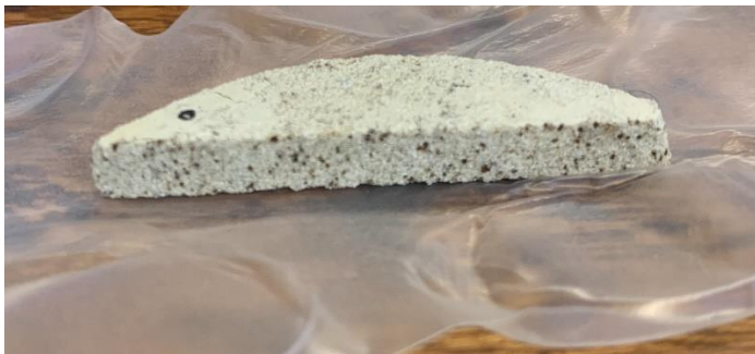
Figure 31. Cut face of a sandstone core sample permeated with gel and subsequently dried. Black marking denotes the surface from which the gel was permeated from.
