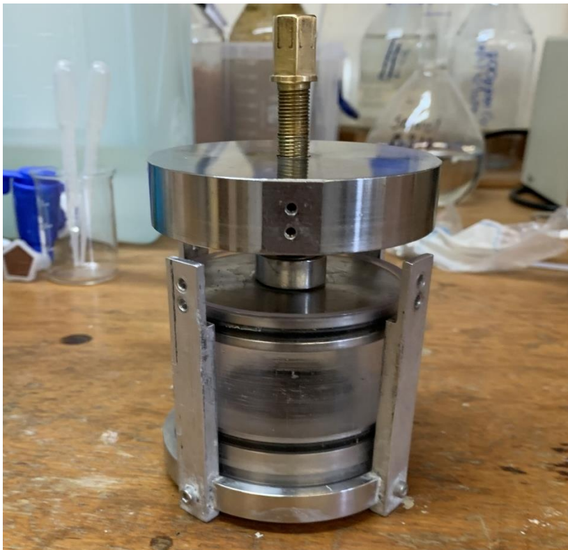
Figure 11. Cylindrical press apparatus used to permeate the gel into sandstone cores.
