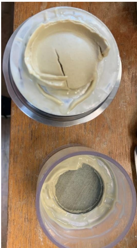
Figure 14. Example of a filter cake formed during permeation of a bentonite gel with the use of the novel apparatus.
