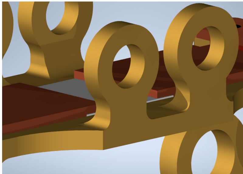
Figure 8.8: Current leads for a short sample, showing the joint between the copper and the CC.
