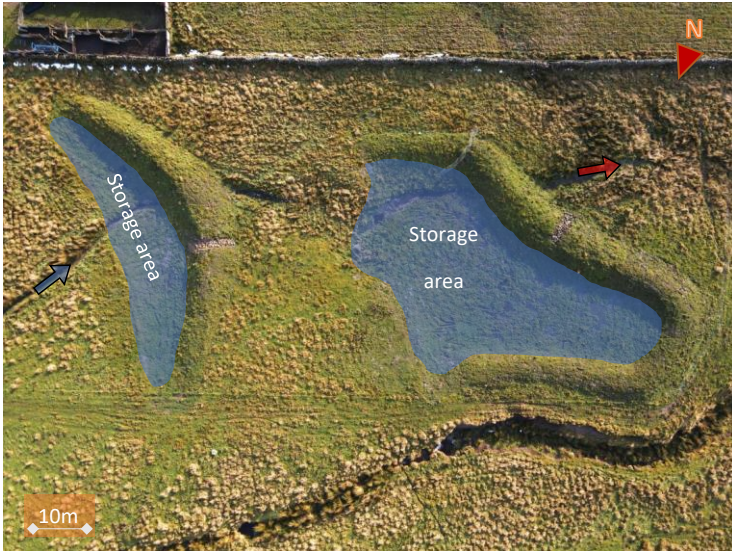
Figure 8. Aerial view of Bunds M16 (left) and M11 (right) (see Fig.4 for location). The inflow via a drainage ditch is indicated by the blue arrow, and the outflow is indicated by the red arrow.
