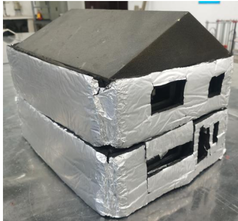
Fig. 5.10 3D printed house model with insulation cotton.
