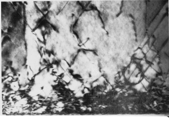
Figure 5.38 — An XTEM micrograph of a Cd 0.06 Zn 0.94 Te epilayer illustrating the dense array of misfit dislocations at the interface
