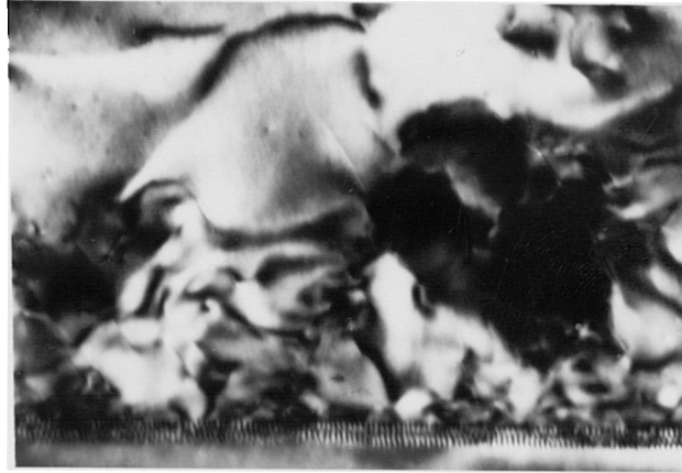
Figure 5.38 — An XTEM micrograph of a Cd 0.06 Zn 0.94 Te epilayer illustrating the dense array of misfit dislocations at the interface
