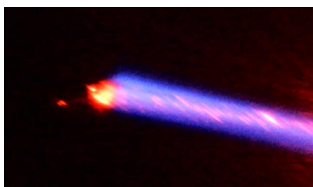
Figure 3.10: USB microscope image of a sample surface with \omega_1 , \omega_2 and \omega_{\text{pump}} present, showing the spot shape, spatial overlap of the beams and bulk fluorescence caused by the pump.
