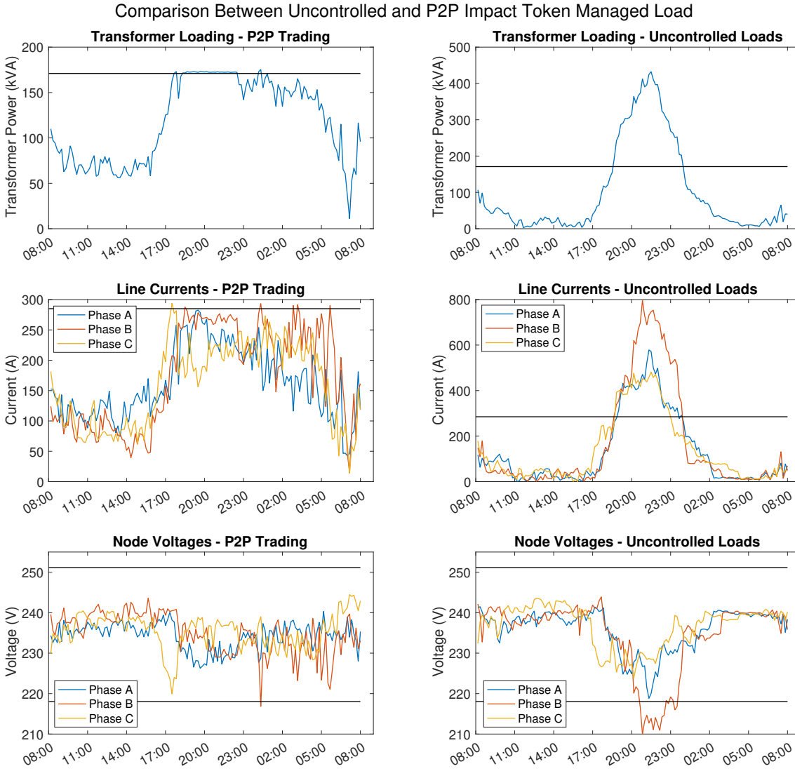
Figure 4.8: A comparison of the transformer loading, line currents and node voltages between the P2P trading of Impact Tokens and uncontrolled loads and generation, showing the importance of managing load in a network
