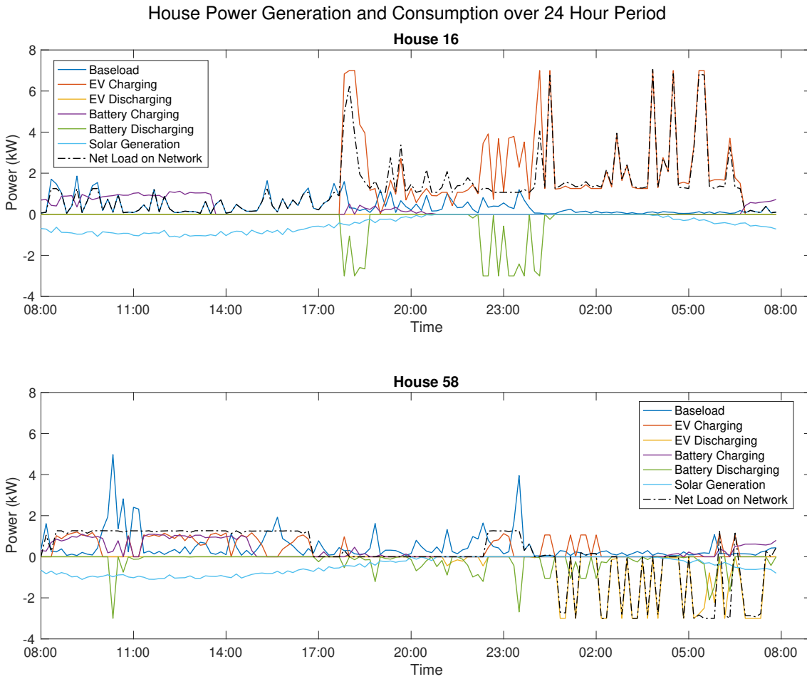
Figure 4.10: Power generation and consumption for two individual houses showing the different load profiles achieved through the P2P trading of Impact Tokens
