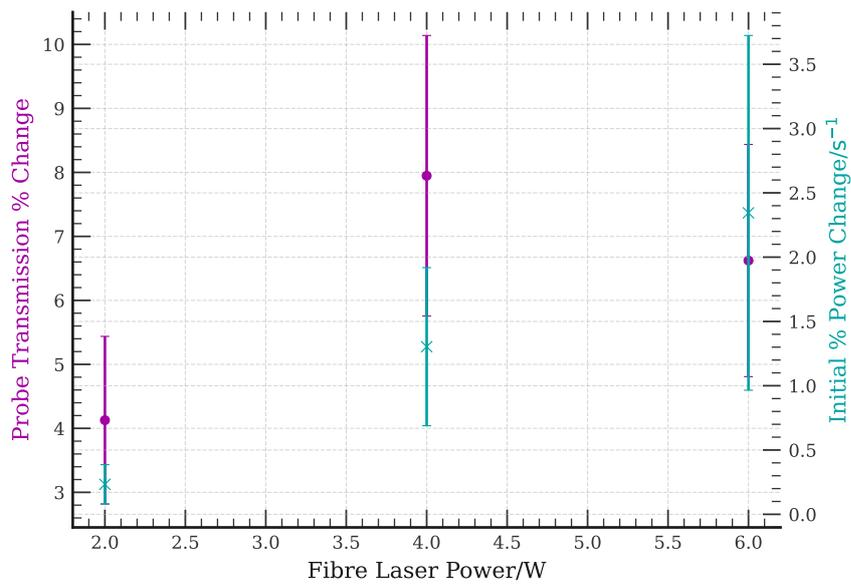
Figure 3.22: Ablation beam power vs probe transmission percentage change (purple) and initial rate of change (blue). Though there is a distinct positive effect in the initial increase of fibre laser power from 2 W to 4 W, the increase from 4 W to 6 W yields no distinguishable improvement.
