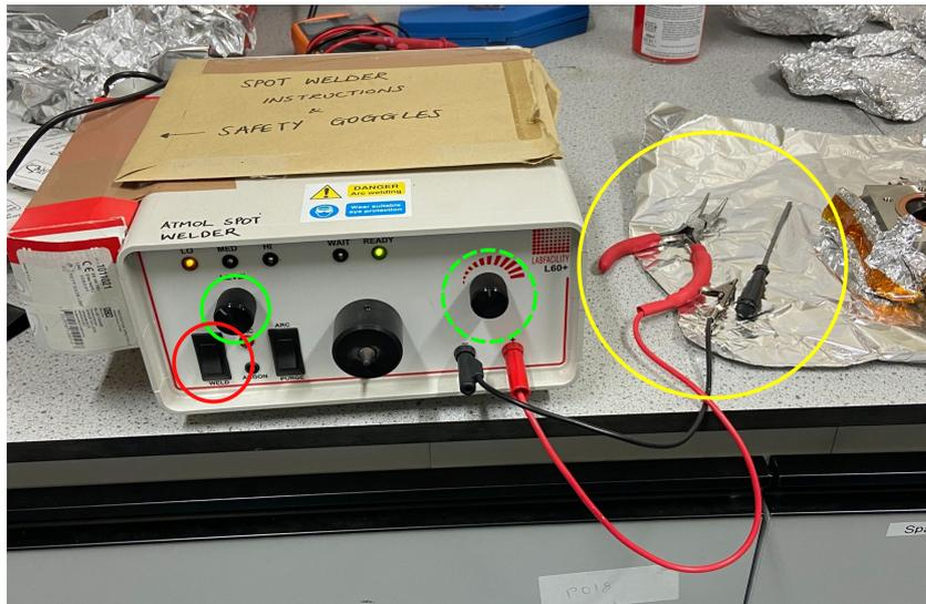
Figure A.3: Spot welder used for the welding described in section 3.3. From left to right, the circled components are the weld switch (red), coarse (solid green) and fine (dashed green) power adjustment knobs and the crocodile clips and pliers for welding (yellow).
