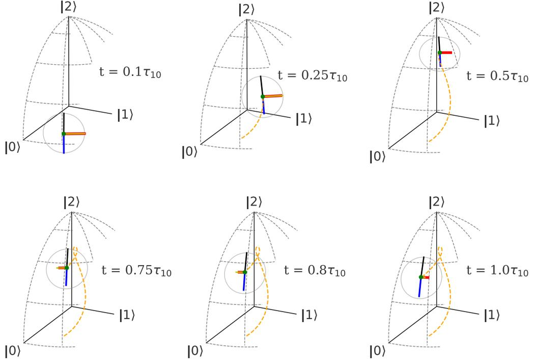
Figure 4.12: Initial dynamics of a FWM process with Rabi frequencies as indicated in the 'Write' stage of figure 4.11. The system begins with an excitation of the qutrit to a long-lived upper state  $|2\rangle$ . The dotted orange line shows the path traced out by the population vector throughout the write sequence.
