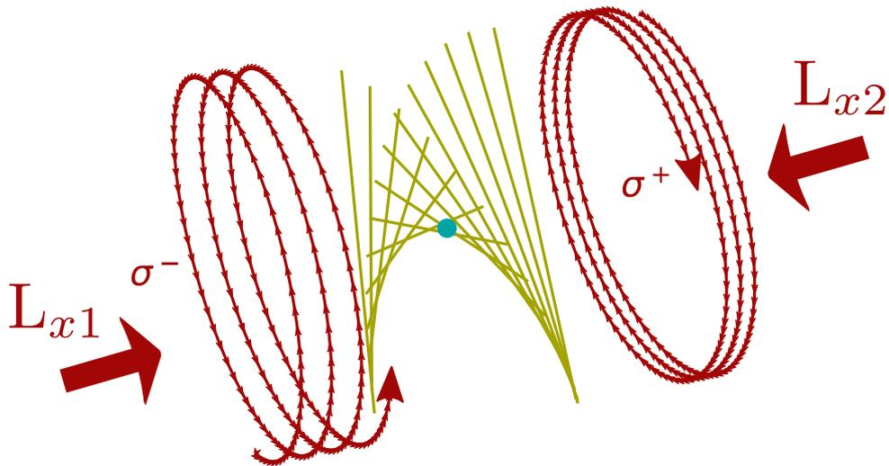
Figure 2.6: Diagram showing the radiation field generated by antiparallel  $\sigma^+$  and  $\sigma^-$  laser beams. The gold lines show the linear polarisation of the radiation field experienced by the atom (cyan).
