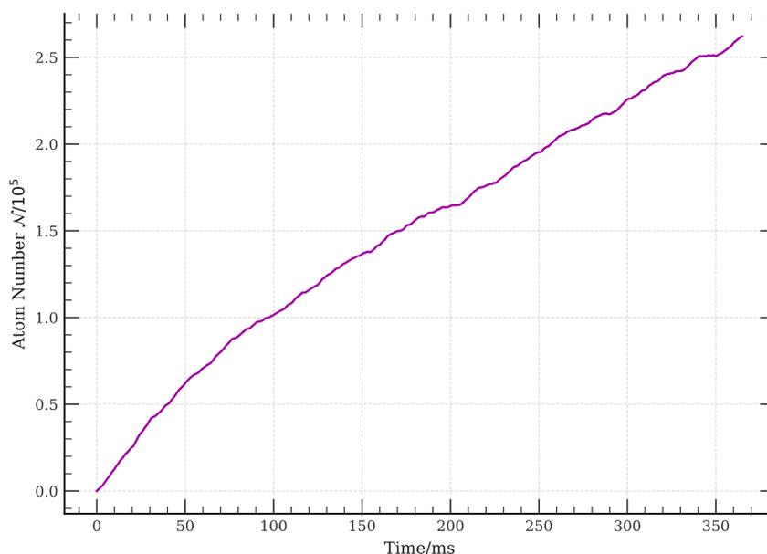
Figure 3.26: Example atomic loading rate over time in a 3D MOT.
