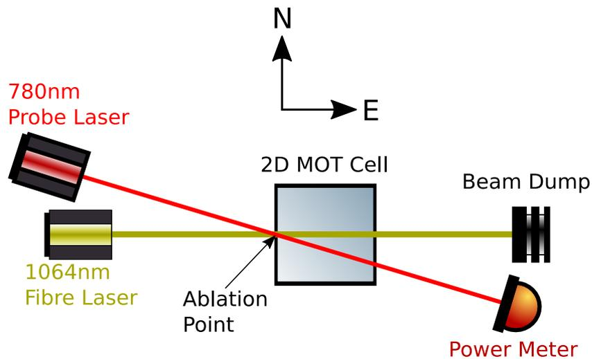
Figure 3.20: Beam diagram for laser ablation. Here, the fibre laser and probe were aligned using the fibre laser’s low-power red guiding beam such that both beams passed through the same spot on the near side of the 2D MOT cell. The high power beam was then dumped and the transmission of the probe over time was recorded on a Throlabs PM100D power meter. When the ablation beam was turned on, the transmission through the cell over time was recorded.
