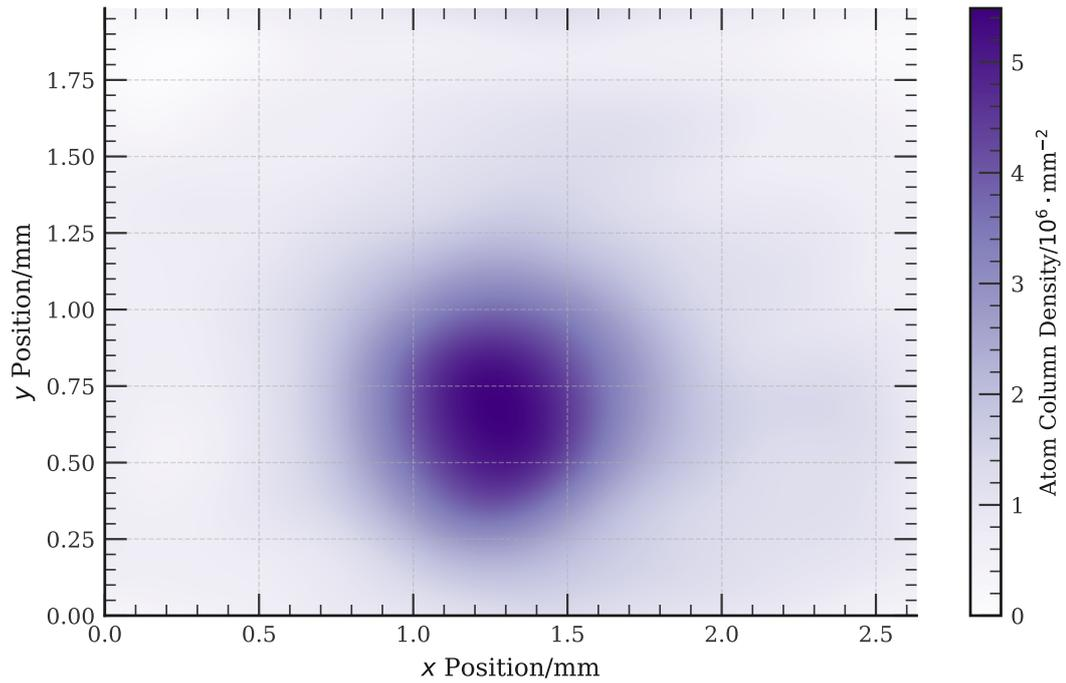
Figure 3.30: Example post-processing absorption image. Co-ordinate axes and number densities have been scaled to account for the magnification of the imaging system.
