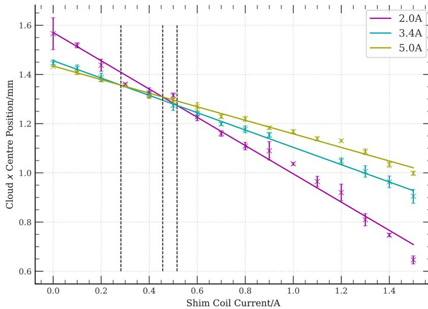
Figure 3.31: Shim Coil Current Optimisation in the East-West direction for anti-Helmholtz MOT coil currents: 2.0 A (purple), 3.4 A (cyan) and 5.0 A (gold). The dashed black lines show the crossing points of the fitting lines used to calculate the optimal value, taken as an average over all three points. In the east west direction, this is  $I_{\text{Opt-EW}} = 0.42 \pm 0.1$  A.
