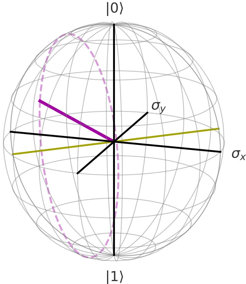
Figure 4.2: Example of a qubit rotation around the Bloch sphere for the test Hamiltonian given in (4.12) with  $\Delta = 0.2 \Omega$ . Here, the solid purple line shows the initial Bloch vector for the density matrix in (4.4a), the dashed purple line shows the path it traces as the system evolves in time and the gold line shows the rotation axis defined by the Hamiltonian.
