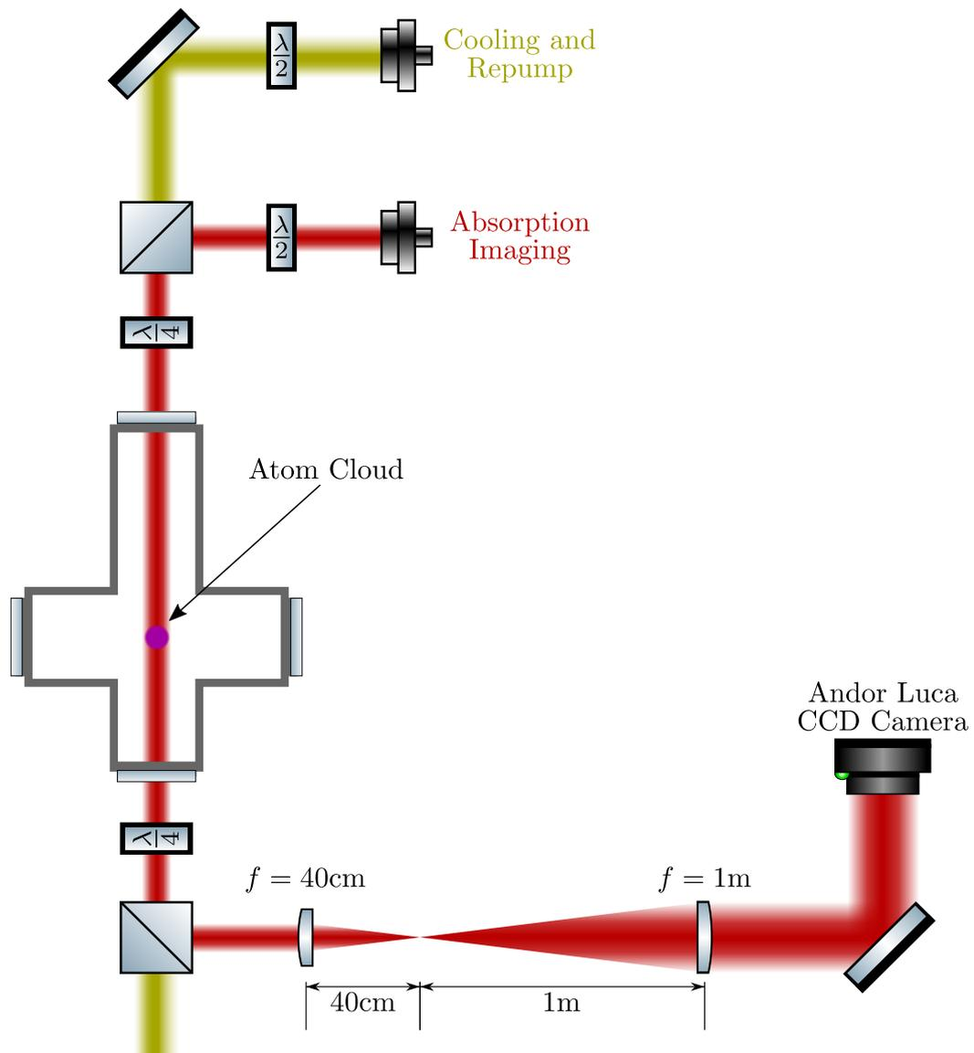
Figure 3.28: Beam diagram for the absorption imaging setup used to characterise MOT position and temperature.
