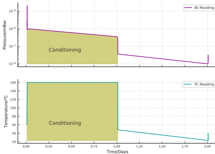
Figure 3.10: Pressure (upper) and temperature (lower) vs time during the first conditioning cycle. The conditioning cycle is highlighted in gold and the activation process is present as the small spike in pressure and temperature after 2 days.
