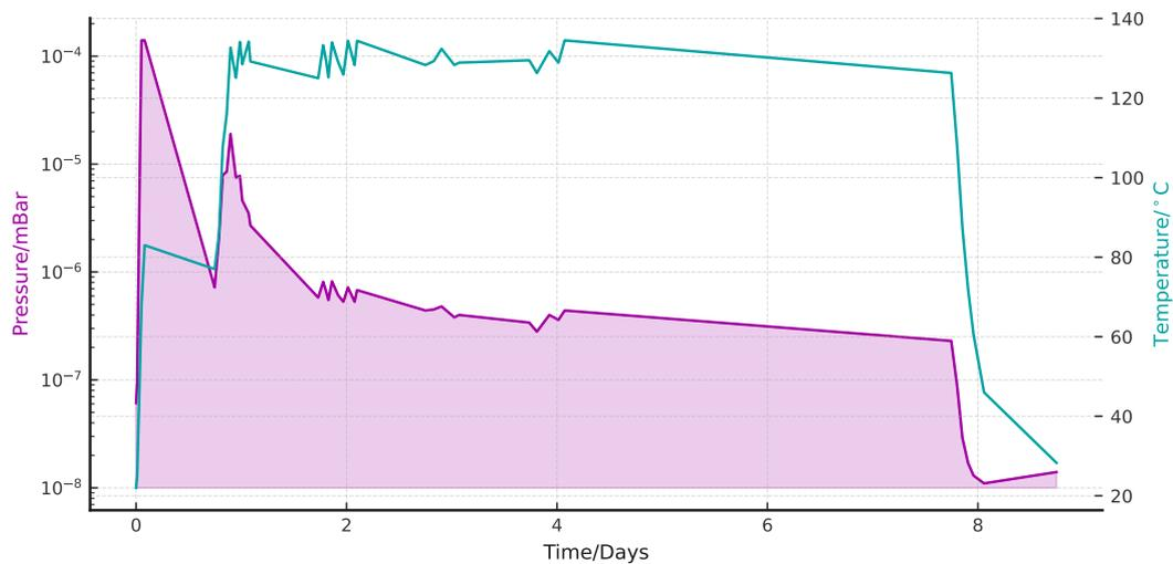
Figure 3.16: Pressure and temperature vs time graph for bake out period. Here, the temperature was held at 135 °C for the majority of the bake due to the  $\sim 5$  °C oscillation around the set temperature of the oven. The initial pressure spike can be attributed to the external vacuum equipment outgassing adsorbed particles after a long period without use.
