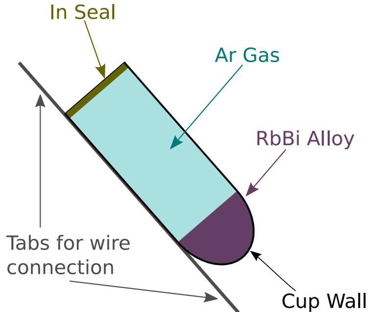
Figure 3.17: Diagrammatic cross section of a dispenser used in the vacuum setup. The Rubidium-Bismuth alloy reacts to release a Rubidium vapour. Due to the rapid oxidisation of the alloy when exposed to atmosphere, the dispensers are manufactured with an Indium seal, sealing a small quantity of inert Argon into the cup.
