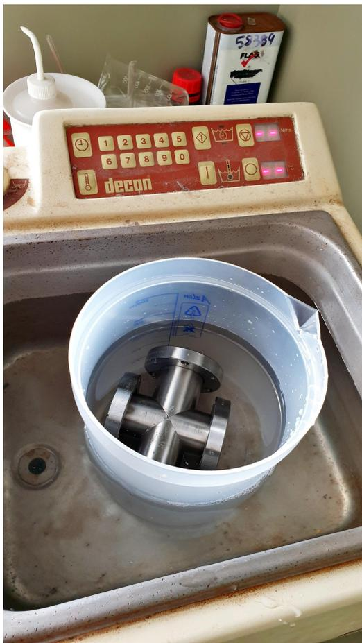
Figure 3.11: The replacement component for the gate valve between the upper and lower chambers of the experiment in the ultrasonic bath for cleaning. The motivation for its inclusion is detailed in section 3.3.5.
