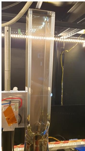
Figure 3.19: Picture of the Rb deposits on the interior walls of the 2D MOT cell. Though the cell can still be seen through by eye, the transmission of a weak probe beam was attenuated by 60% in the worst affected areas.
