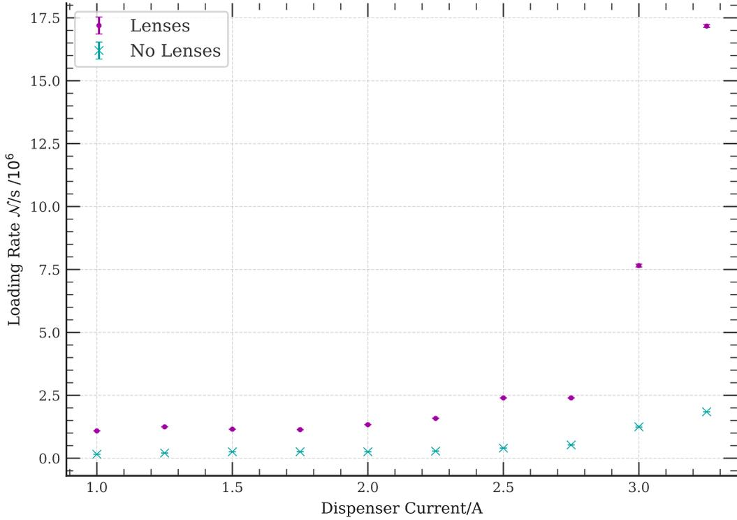
Figure 3.27: 3D MOT loading rates vs dispenser current both with (purple) and without (cyan) focusing optics. Errorbars shown here are derived from the numerical errors on the fitting parameters in (3.7).
