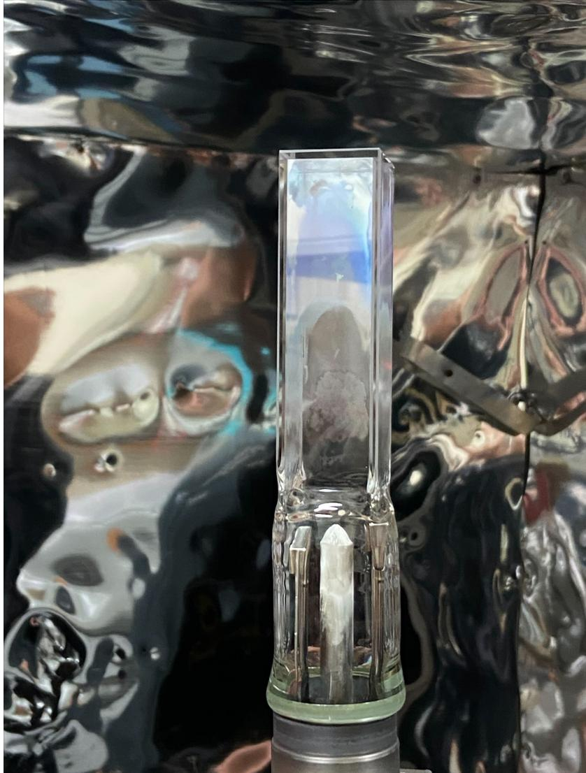
Figure 3.25: Blue residue deposited on the interior lining of the 2D MOT cell for the second dispenser activation.
