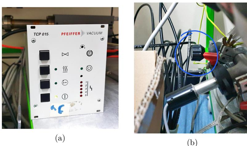
Figure A.2: Turbo pump power supply (a) and gate valve (b) circled in blue.
