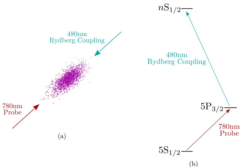
Figure 2.11: A weak 780nm probe beam excites an unspecified atom in an atomic cloud to state  $5P_{3/2}$  whilst being illuminated by a coupling beam addressing the transition  $5P_{3/2} \rightarrow n_{1/2}$ . **(a)** shows the two counter-propagating beams addressing the atomic cloud and **(b)** shows the energy level diagram of the process.
