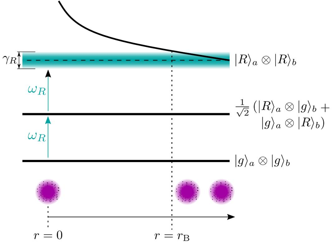
Figure 2.9: The Rydberg blockade mechanism. The van der Waals interaction of the existing Rydberg atom ( $|R\rangle_a$ ) shift the excitation energy required to generate a second ( $|R\rangle_b$ ). At distances from the first Rydberg atom  $r < r_B$  this energy shift (solid black) is greater than the excitation laser's ( $\omega_R$ ) linewidth ( $\gamma_R$ ), thus no additional Rydberg atom can form within this radius.
