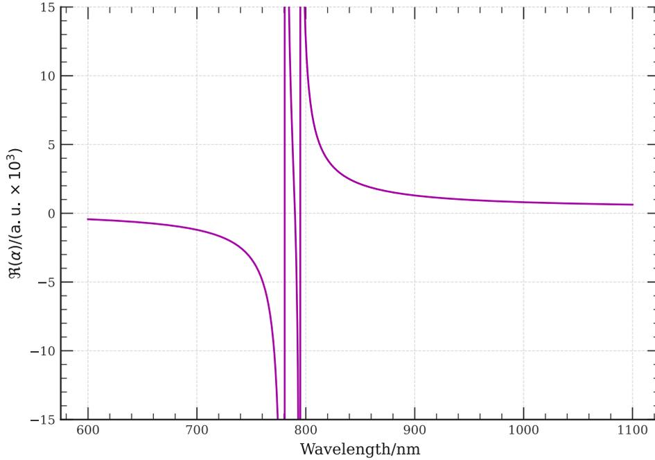
Figure 2.7: Real part of the polarisability  $\alpha$  for  $^{87}\text{Rb}$  for both the  $D_1$  (on the right, at 794.978 nm) and  $D_2$  (on the left, at 780.241 nm) transitions. The conversion between atomic (a.u.) and S.I. units is given as  $\Re(\alpha)_{\text{a.u.}} = \Re(\alpha)_{\text{S.I.}} / (4\pi\epsilon_0 a_0^3)$
