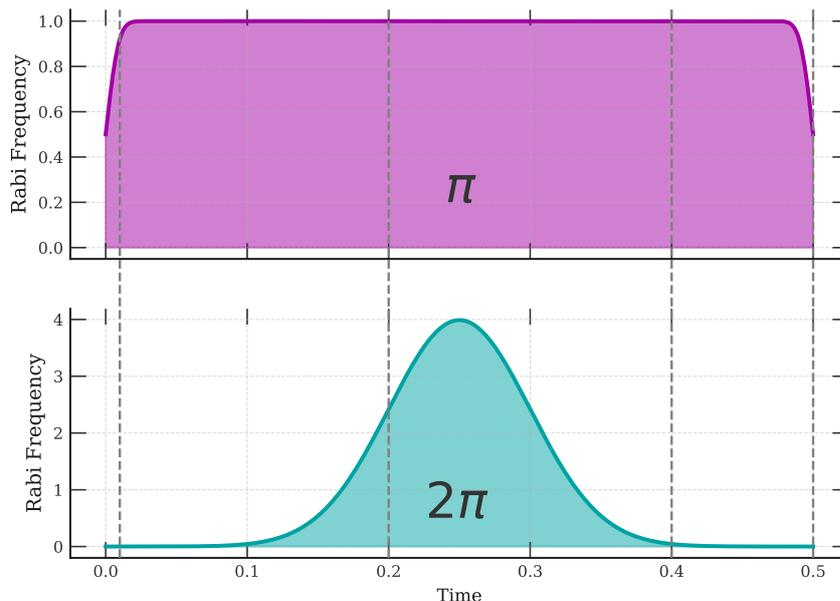
Figure 4.6: Pulse sequence for a simple simultaneous excitation scheme. A  $\pi$  pulse is applied to address the  $|0\rangle \rightarrow |1\rangle$  transition (blue), and is applied weakly such that the pulse take the entire duration of the sequence to execute. Simultaneously to this, a stronger  $2\pi$  pulse addresses the  $|1\rangle \rightarrow |2\rangle$  transition (gold) with a Gaussian intensity profile. The grey dashed lines mark the times with corresponding octant plots in figure 4.7.
