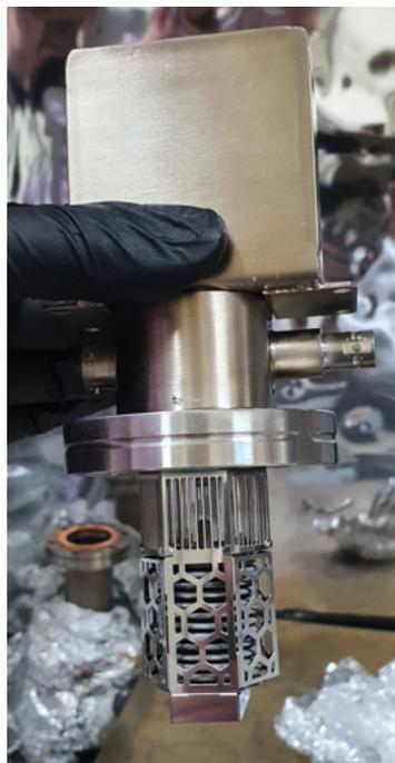
Figure 3.8: NEX Torr SIP and NEG elements.
