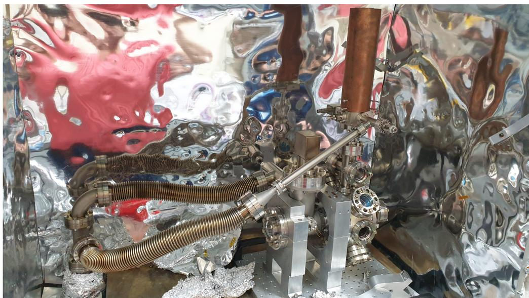
Figure 3.13: Experimental Vacuum Chamber in bakeout oven, attached to the external pumping rig. The connection from the pumps is made using two sets of bellows attached via DN40 flanges (bottom left) and attaches to the chamber via gate valves on both the upper and lower chambers. The aforementioned pumps are not pictured here and are sat beneath the oven.
