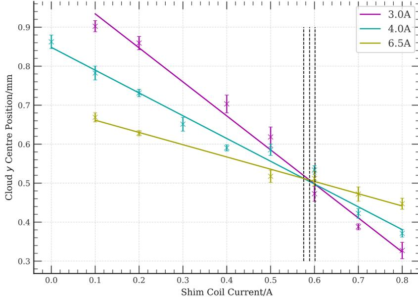
Figure 3.32: Shim Coil Current Optimisation in the Up-Down direction for anti-Helmholtz MOT coil currents: 3.0 A (purple), 4.0 A (cyan) and 6.5 A (gold). The dashed black lines show the crossing points of the fitting lines used to calculate the optimal value, taken as an average over all three points. In the up-down direction, this is  $I_{\text{Opt-UD}} = 0.59 \pm 0.01$  A.
