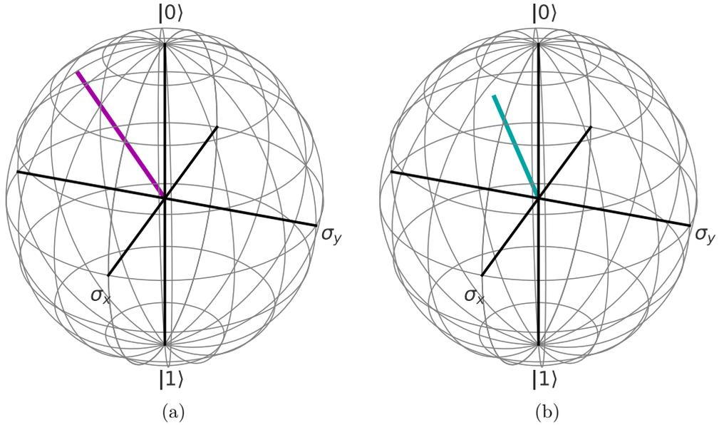
Figure 4.1: Bloch vectors for the pure (a) and mixed (b) qubit states given in (4.4a) and (4.4b).
