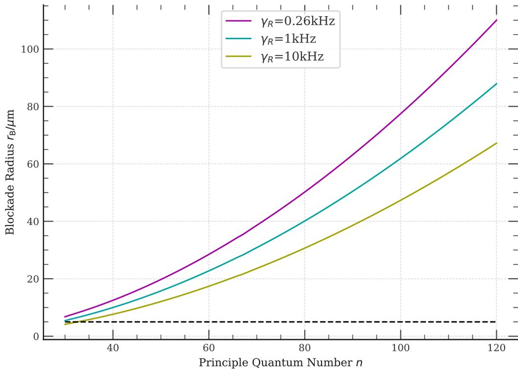
Figure 2.10: Principle quantum number vs blockade radius for excitation laser linewidths of 0.26 kHz (purple), 1 kHz (cyan) and 10 kHz (gold). The dashed black line shows the radial  $1/e^2$  diameter of the 852 nm tweezer trap. The lower linewidth limit defined by the purple line is taken from [115].
