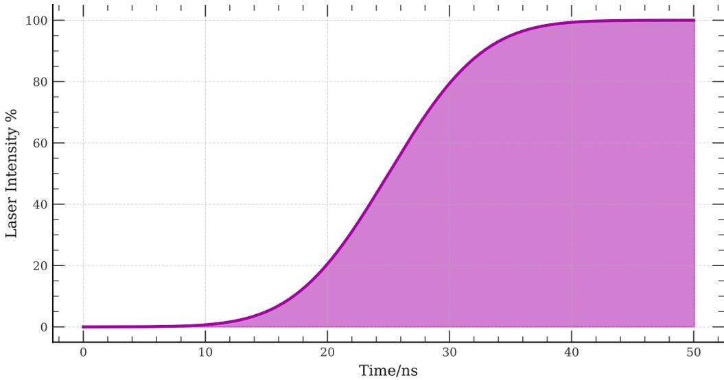
Figure 3.3: Example AOM intensity change for a rise time  $r_{10:90} = 10$ ns.
