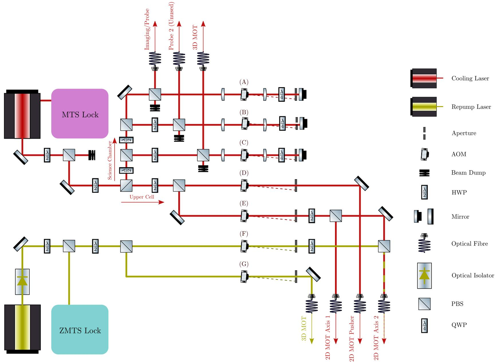
Figure 3.1: Beam diagram showing the optical setup of the cooling and repump lasers. The Acousto-Optic Modulator (AOM) channels (A-G) shown here correspond to those listed in figure 3.4.
