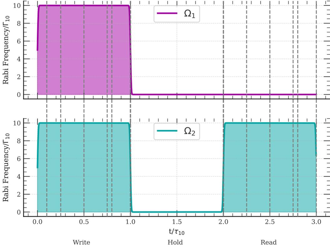
Figure 4.11: Rabi frequencies of the probe and coupling beams in a resonant FWM process. The grey dashed lines show the times during the write (read) stage that are shown in figure 4.12 (4.13).
