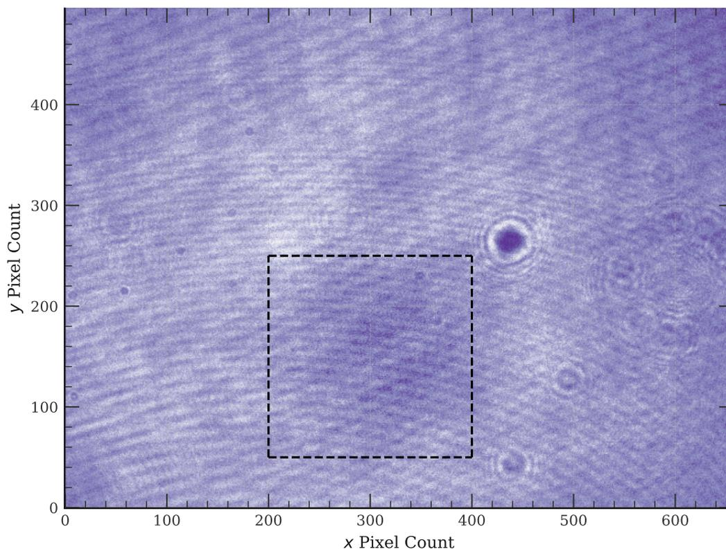
Figure 3.29: Example intensity noise in a background subtraction of an image with a MOT present from one with no MOT present. Later analysis reveals that the ROI outlined in black dashed lines is the MOT image.
