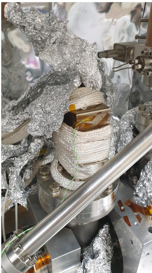
Figure 3.9: Ion pump conditioning setup with heater tape and control thermocouples.
