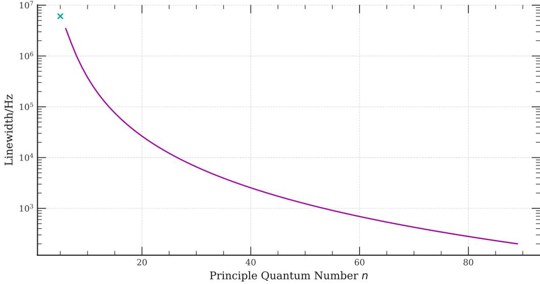
Figure 3.2: Principle quantum number  $n$  vs linewidth  $\Gamma_n$  of transition  $|5P_{3/2}\rangle \rightarrow |nS_{1/2}\rangle$ . The cyan cross in the top left of the plot shows the linewidth of the  $|5P_{3/2}\rangle$  state. Values of linewidths were obtained using the ARC python library [130].
