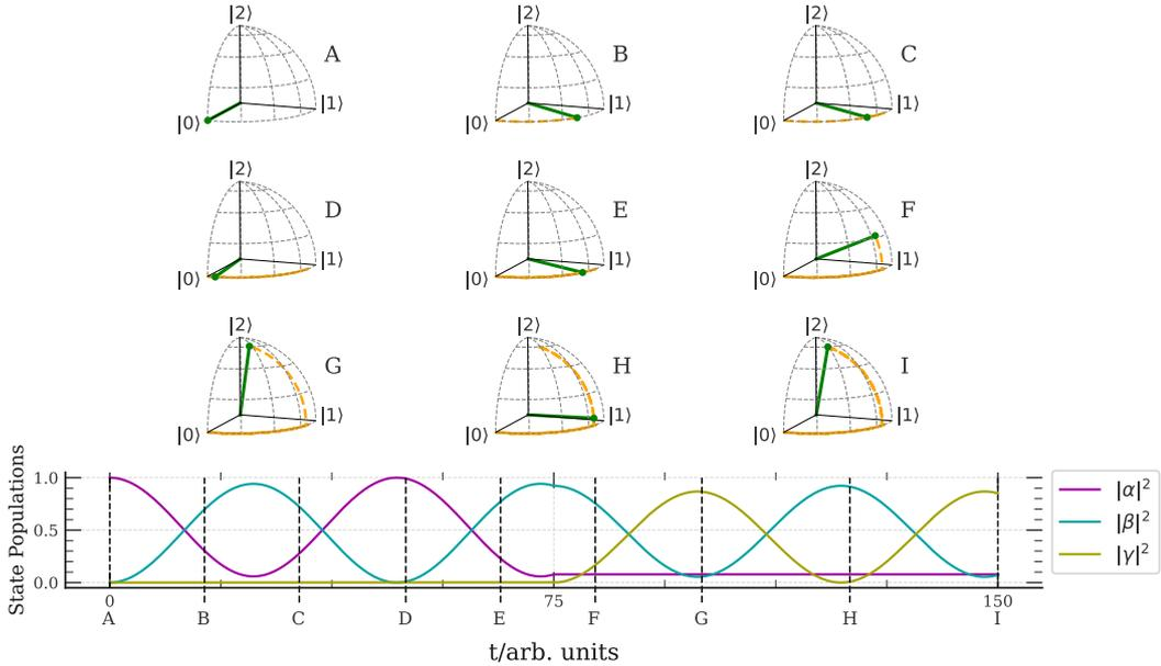
Figure 4.4: **Upper:** Octant plots displaying Rabi oscillations in a 3 level system. No clock hands are included here due to the lack of any oscillation or decay in the resonant case free of decay modes. **Lower:** A more traditional state population vs time evolution of the qutrit as a reference. The times where octant plots are drawn are marked with lettered black dashed lines.
