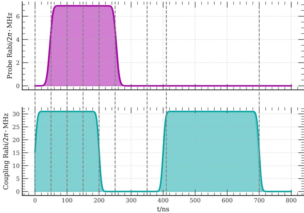
Figure 4.14: Pulse sequence for the simulated Rydberg atom formation. In line with section 2.3.2, the probe beam is switched on and off after the equivalent steps for the coupling beam to ensure that any atom that is excited to the  $5P_{3/2}$  state is further excited to the  $6S_{1/2}$  state. The grey dashed lines shown here denote the times where octant plots are shown in figure 4.15.
