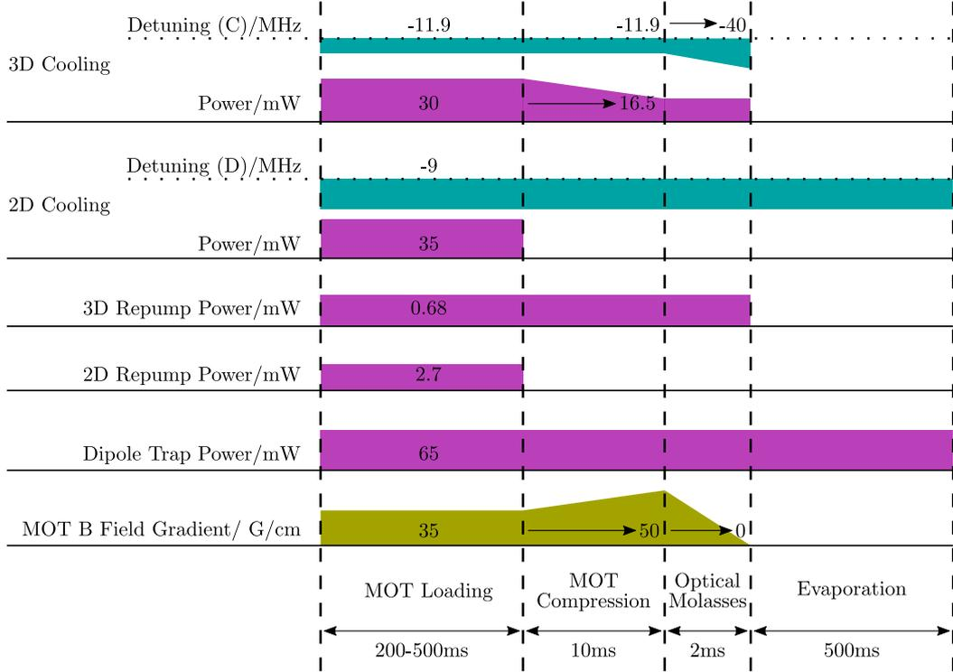
Figure 3.35: Laser intensities (purple), detunings (cyan) and field gradients (gold) throughout an experimental sequence. The lettering (C-D) correspond to that in figures 3.1 and 3.4. The sequence used to prepare the clouds shown in figure 3.33 is identical to this one except instead of an evaporation stage, the two pulses of the imaging beam are triggered with a separation of 50ms to allow the MOT cloud to dissipate.
