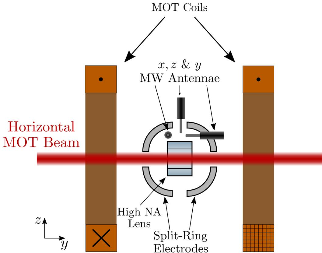
Figure 3.7: Cross section of the science chamber in the  $y - z$  plane showing *in-vacuo* components. Adjacent to each high NA lens is a quartet of DC split-ring electrodes (for a total of eight). Between the lenses are a set of three microwave stub antennae designed for a frequency range of DC – 40GHz. The rectangular MOT coils are shown in copper-orange, with the bottom right cross section split to show the  $8 \times 7$  grid arrangement of the coils.
