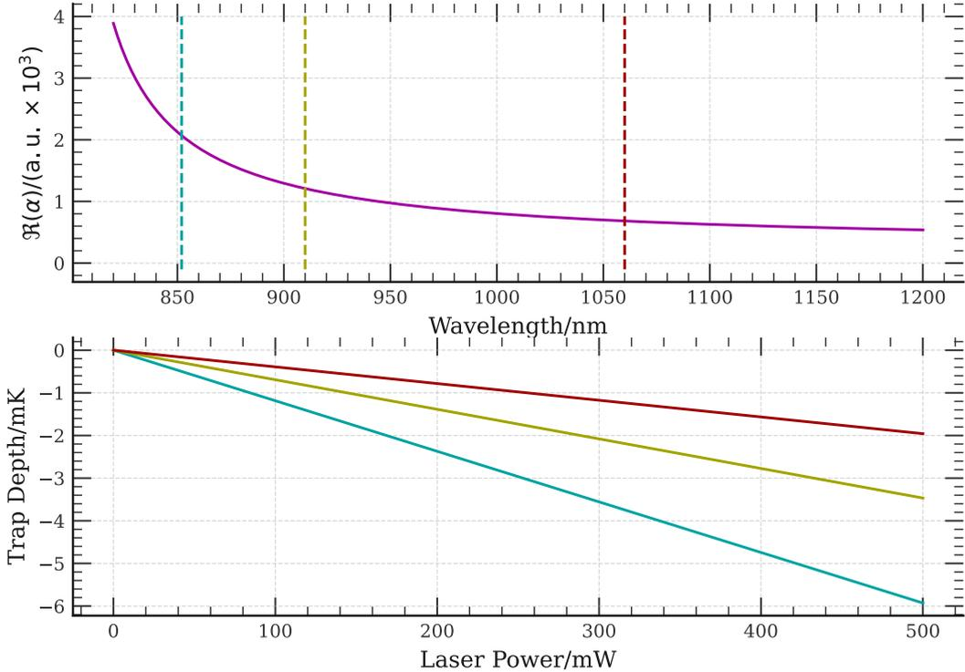
Figure 2.8:  $\Re(\alpha)$  vs wavelength for  $\lambda > 820$  nm (upper) and trap depths for past and present dipole trap wavelengths (lower) with a  $5\mu\text{m}$  beam waist. The 910 nm (gold) and 1080 nm (burgundy) traps were used in previous iterations of the experiment and the 852nm (cyan) trap is currently utilised. The dashed lines in the upper plot correspond to wavelengths shown in the lower plot.
