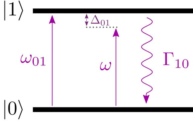
Figure 2.1: Energy level diagram showing two levels  $|0\rangle$  and  $|1\rangle$  separated by an energy  $E_{01} = \hbar\omega_{01}$ , driven by a laser field of energy  $E = \hbar\omega$ , detuned below resonance by  $E_{\Delta} = \hbar\Delta_{01}$  and with a decay mode from  $|1\rangle \rightarrow |0\rangle$  at a rate of  $\Gamma_{10}$ .
