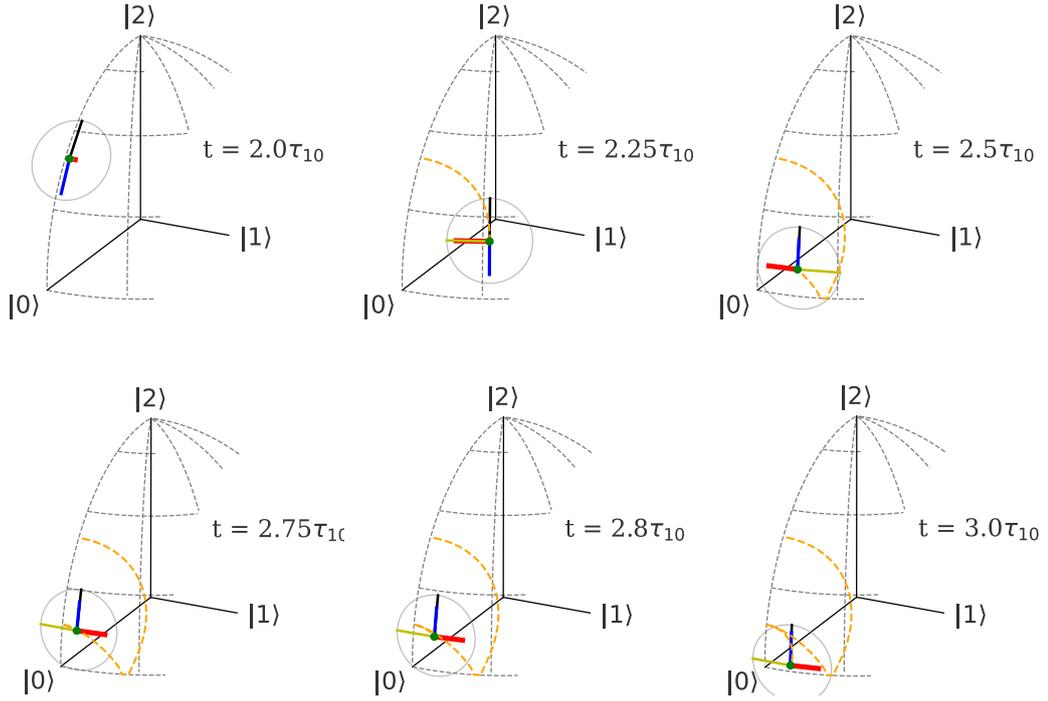
Figure 4.13: End of the FWM process described. Here, the qutrit de-excites from  $|2\rangle$  state to the ground state via a strongly decaying intermediate state. The starting state shown here is different from the end state in figure 4.12 as an additional  $\tau_{10}$  has passed between the two figures, causing the residual population in  $|1\rangle$  to decay. The dotted orange line shows the path traced out by the population vector throughout the read sequence.
