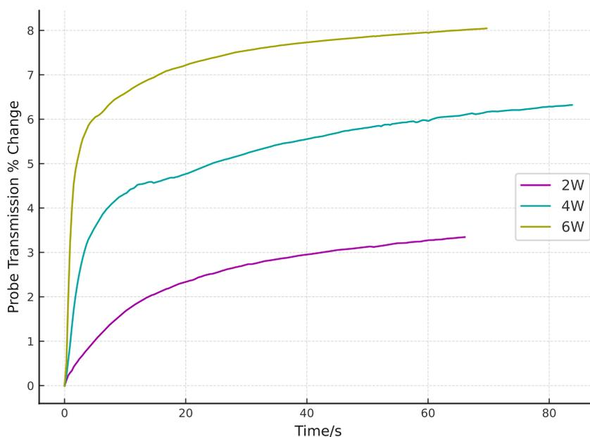
Figure 3.21: Example probe transmission change through the 2D MOT cell during the ablation process. Time  $t=0$  is set to when the high-power beam is switched on. A case where all three curves are distinguishable is shown here, however this was not generally the case, and a substantial variation in efficacy for different beam powers was observed. This effect is illustrated in figure 3.22.
