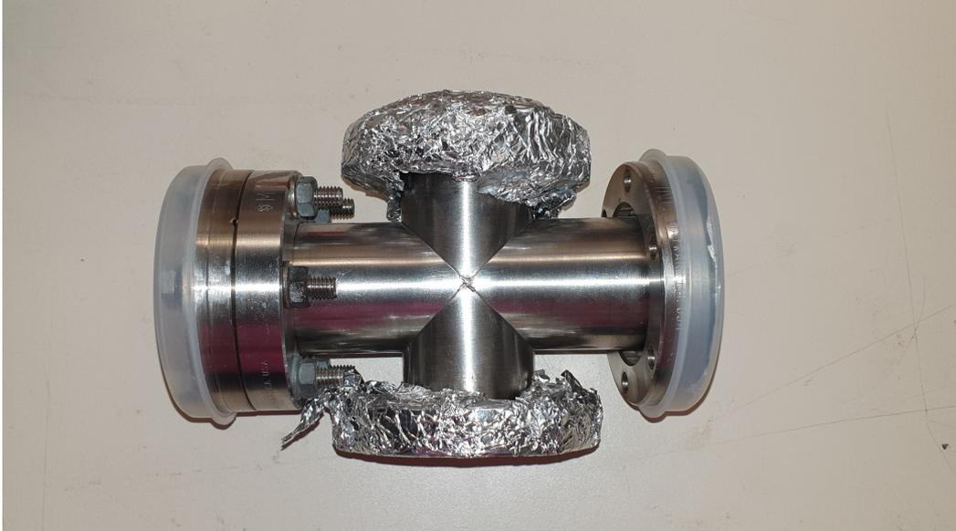
Figure 3.12: Cross piece added to vacuum chamber in place of a gate valve. The longer axis was used to connect the chambers and the shorter axis had viewports (AR coated at 780nm) added for incorporation of a weak probe for future atomic beam density and temperature measurements.
