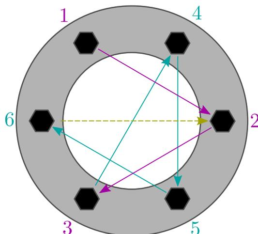
Figure 3.14: Tightening procedure for a standard DN16/ DN40 flange to ensure even pressure distribution throughout. The bolts are tightened in two sets of triangles (purple then teal), with the first bolt of the second three being the one directly opposite the last one of the first three. This pattern then continues round (gold) until no further tightening can be achieved.
