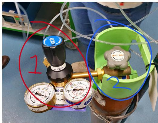
Figure A.6: Valves of the He canister with a regulator valve attached.
