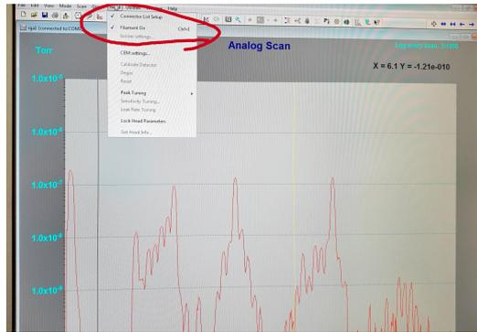
Figure A.5: Connector List Setup under Head dropdown menu.
