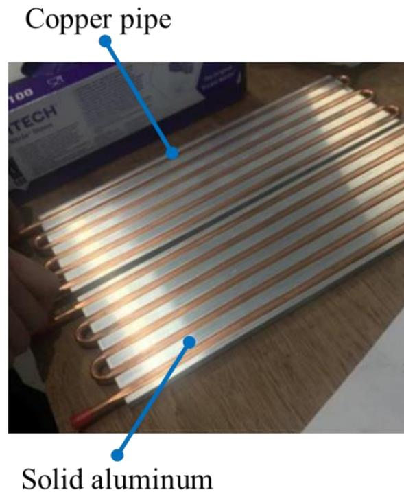
Fig. 4.6 Photo of the battery cooling module.
