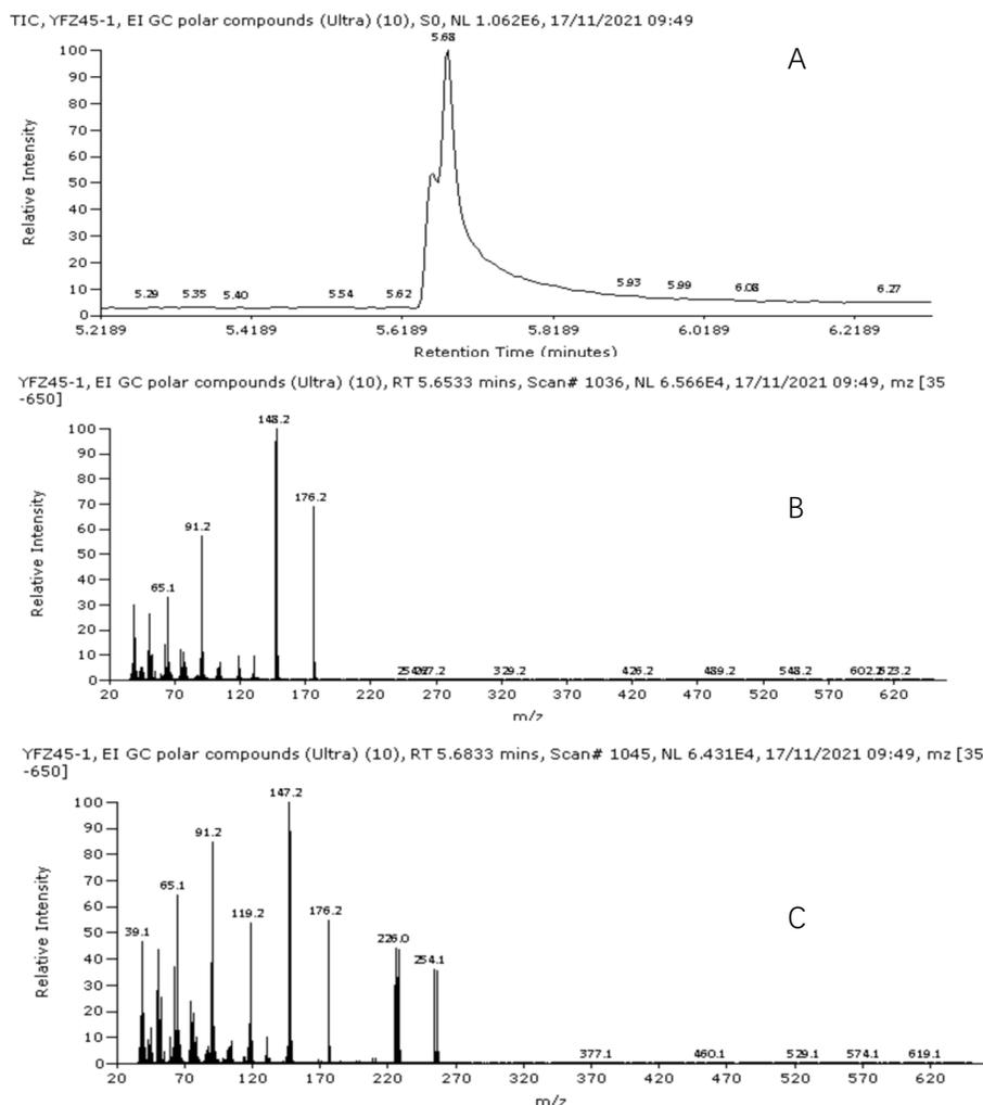
**Figure 24.** The GC-MS analysis of 6-bromo-4-methyl-7,8-dihydro-2*H*-chromene-2,5(6*H*)-dione (**44**). **A** The detected peaks at retention time. **B** The molecular ion peak indicating 5-hydroxy-4-methylcoumarin (**46**) at  $m/z = 176.2$ ,  $R_t = 5.65$  min. **C** The molecular ion peak indicating 6-bromo-5-hydroxy-4-methylcoumarin (**44**) at  $m/z = 176.2$ ,  $R_t = 5.65$  min.
