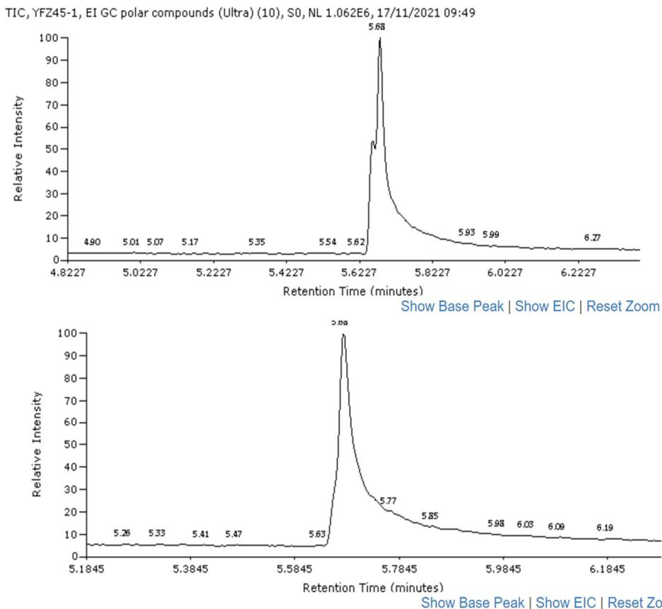
**Figure 26.** The comparison of 6-bromo-4-methyl-7,8-dihydro-2H-chromene-2,5(6H)-dione (**45**) ratio without and with degassing of oxygen in reaction system by GC-MS. For both cases, at  $R_t = 5.68$  min,  $m/z = 254.1$  and  $256.1$ .
