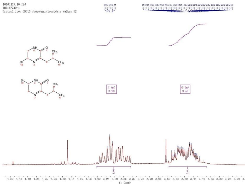
**Figure 30.** The <sup>1</sup>H NMR integral ratio of hydrogens at position 1 and 2 of **63** or **63'** is approximately 2:1 or 1:2.
