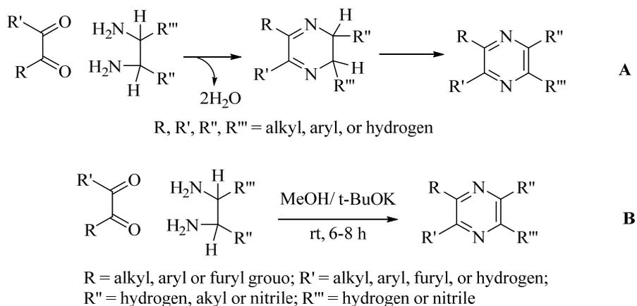
**Scheme 13.** The preparation of alkyl pyrazines through condensation of  $\alpha,\beta$ -diketone and 1,2-diamine by Ghosh *et al.* 2012.<sup>[2]</sup>
