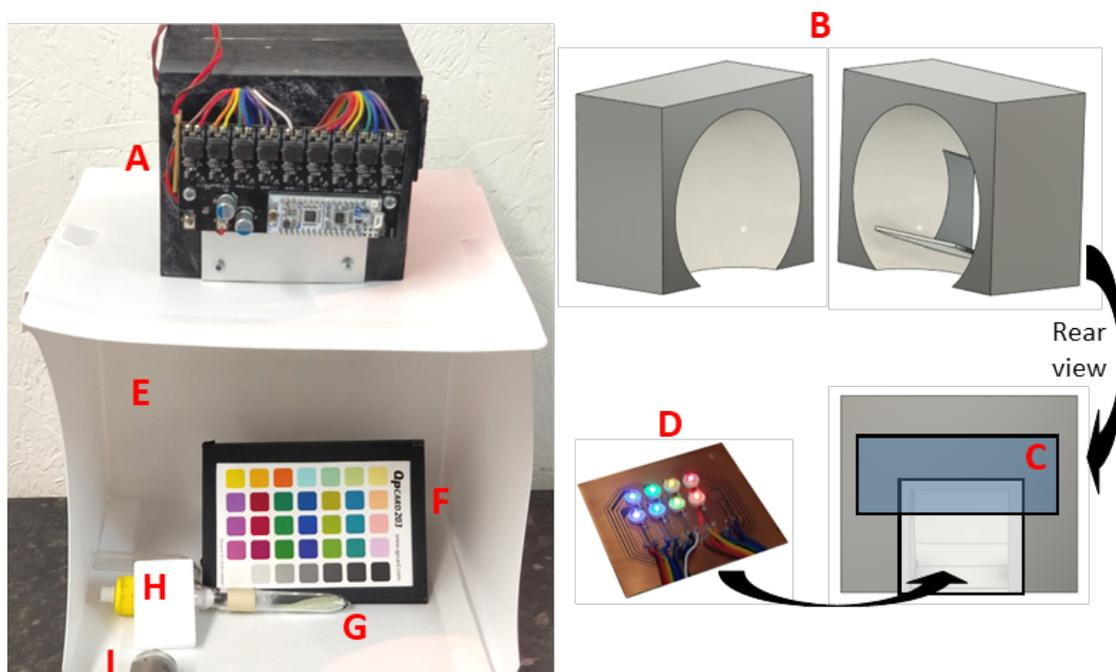
**Figure 2.16** Experimental setup of spectrally tunable light source. A) tunable light source unit comprised of: integrating sphere shown as split halves in CAD model (B), LED array (D) and LED drivers & power control electronics (C). E) Photography enclosure. F) QP 203 colour standard card. G) Anhydrous neodymium chloride sample. H) PTFE diffusely reflective block. I) Collimator fibre-coupled to spectrometer.
