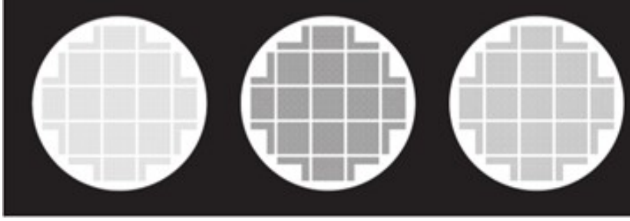
Figure 2.1: Photomasks for developing patterns of cylindrical wells. (left, centre and right are for fabricating wells with radius 75.0\ \mu\text{m} , 30.0\ \mu\text{m} and 50.0\ \mu\text{m} , respectively.)
