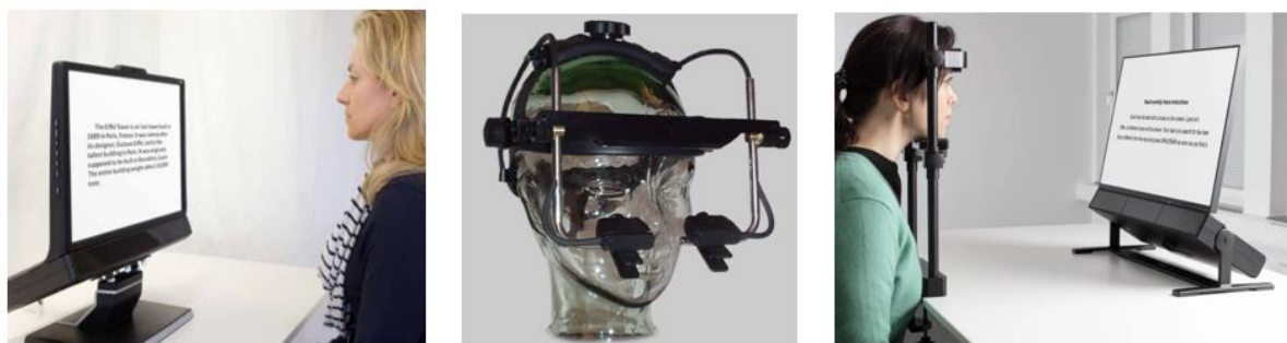
Figure 4-4. Examples of the three types of eye-trackers (a remote eye-tracker on the left, a head-mounted eye-tracker in the middle, and an eye-tracker with a chin-rest on the right)
