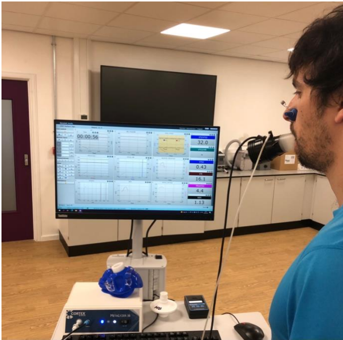
Figure 13: The Hans Rudolph (9060, USA) mouthpiece and nose clip that was used to connect to the turbine and M3B.
