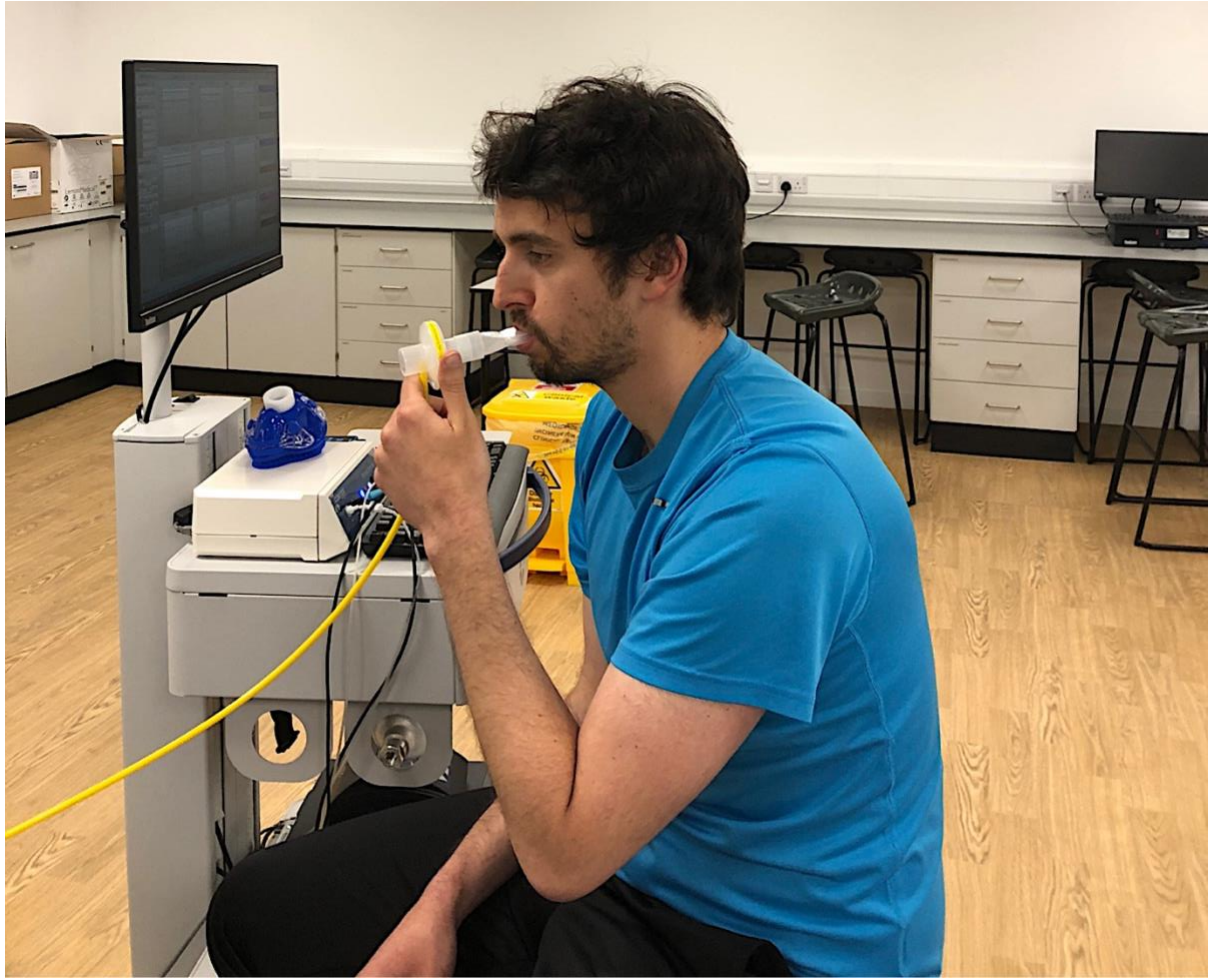
Figure 6: A pilot participant demonstrating how the mouthpiece connects the gas inlet line from the CELIF BrAce detector to the participant's breath.
