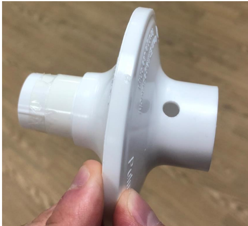
Figure 9: LemonMedical adaptor, which has been adapted through drilling a hole that is identical to the diameter of the gas inlet line from the CELIF BrAce detector.
