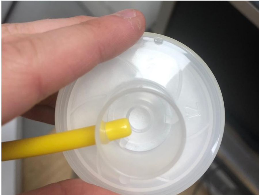
Figure 16: A comparison of the gas inlet line covering and not covering the hole where the acetone from an individual's breath goes. This may impact the amount of the participant's breath goes down the gas inlet line, thus impeding the validity of BrAce detected by the CELIF BrAce detector. Thus, during future data collection, the research team ensured the gas inlet line was just below the hole of the mouthpiece.
