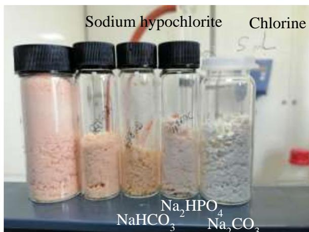
**Figure 25.** Comparison of colours obtained performing basic washings with sat. solution of  $\text{NaHCO}_3$ ,  $\text{Na}_2\text{HPO}_4$  and  $\text{Na}_2\text{CO}_3$  with the white Veramoss (**11**).
