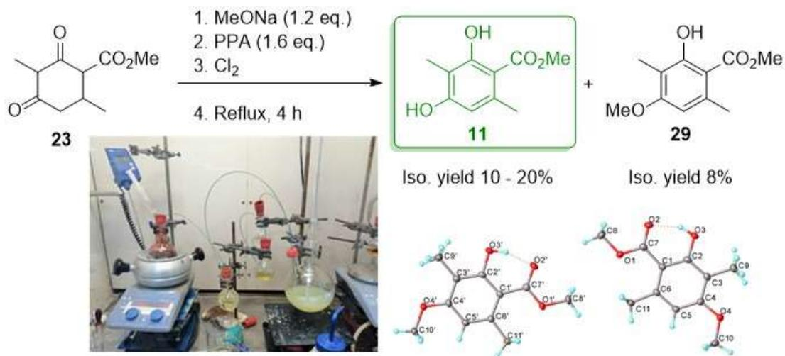
**Scheme 32.** Set-up for the chlorine oxidation of **23**. The reaction formed Veramoss (**11**) and **29** as the major by-product.
