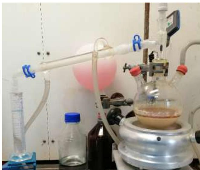
**Figure 38.** Apparatus used for the one-pot procedure of the synthesis of **37**. In the flask two layers can be noticed; the bottom layer is mainly formamide along with  $\text{CaCl}_2$  and the top layer is where the product is distilled from.
