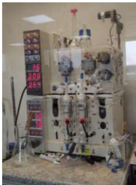
**Figure 51:** Setup for the continuous-flow preparation of the nitro olefin **77**.
