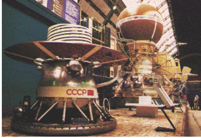
Figure 1.7: Archive photo of the Venera satellite series. The SIGNE-2MS and the KONUS detectors were mounted on the Soviet satellites to search for gamma-ray bursts at the end of the 1970s. Image Credit: NASA, https://heasarc.gsfc.nasa.gov/docs/heasarc/missions/venera1112.html , last accessed on 01/08/22.
