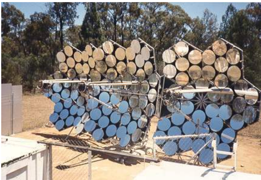
Figure 1.26: Mark III gamma-ray telescope located in Narrabri, New South Wales, Australia. The Mark III consisted of a single mount with three 11\text{-m}^2 reflectors formed from 40+ smaller spherical mirrors made out of anodised aluminium supported by an aluminium honeycomb structure. Image credit: Durham University, Gamma-ray Group, https://www.dur.ac.uk/cfai/vhegammaraygroup/grouphistory/australia/ , last accessed on 01/08/22.
