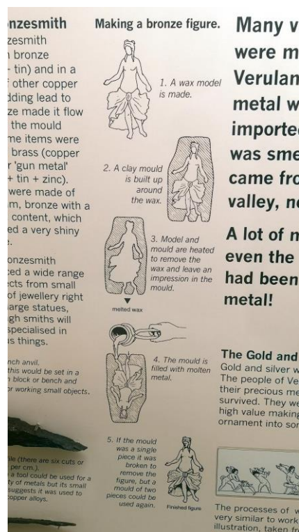
Fig 8.33: Bronze casting process at Verulamium Museum. Author's photograph
