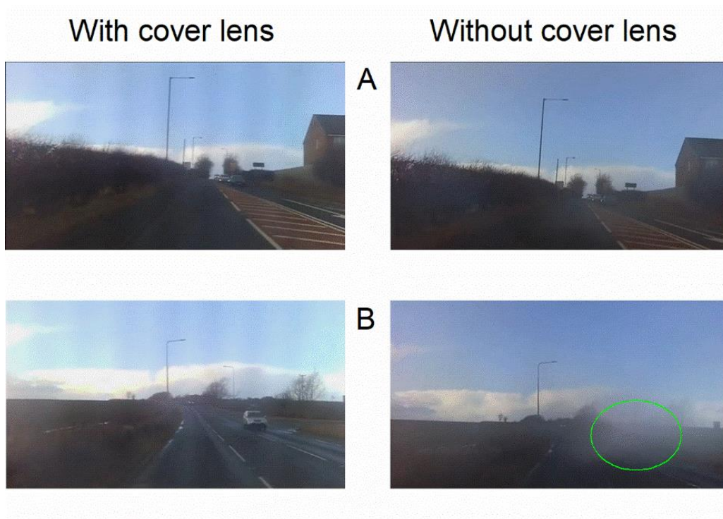
Figure 69 Testing on the road experiment with a vehicle moving at 40 mph. There are two testing cameras, (left) one with a self-cleaning cover lens, and (right) the other one had a standard plastic cover lens. The wind shear force of a moving vehicle prevented any droplet sticking to the camera on the left. However, the camera on the right with a less hydrophobic surface allowed droplets to remain attached the surface (illustrated by a green circle).
