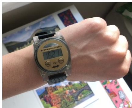
Figure 7. Illustration of Motionlogger Micro Watch units and their size relative to an adult wrist.
