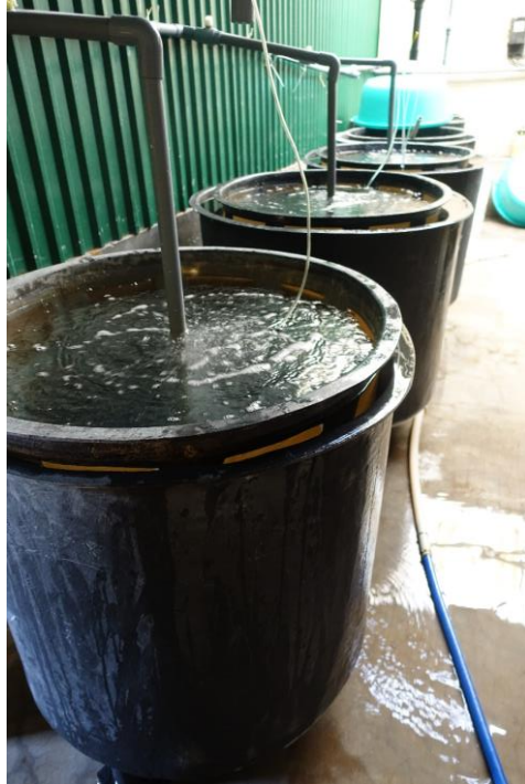
Figure 16 Double washing system to wash away the eggshell and other toxic materials on the body of nauplius
