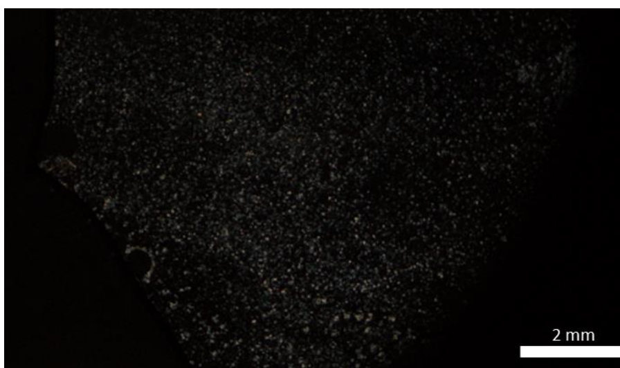
Figure 3.1: AC12 ·BF 4 under POM cooling to a birefringent liquid crystal phase from the non-birefringent isotropic phase.
