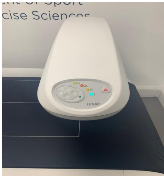
Figure 4. GE Lunar iDXA scanner arm highlighting the control systems to manually position the laser for the DXA scan
