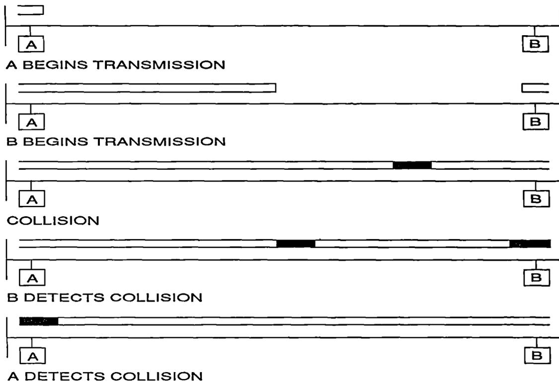
Figure 4 : Carrier Sense Multiple Access Topology
