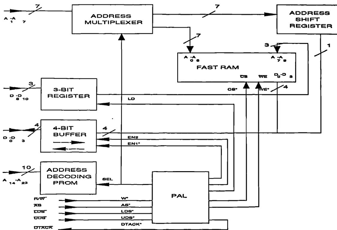
**Figure 16 : Detailed Block Diagram of Transmitter**
