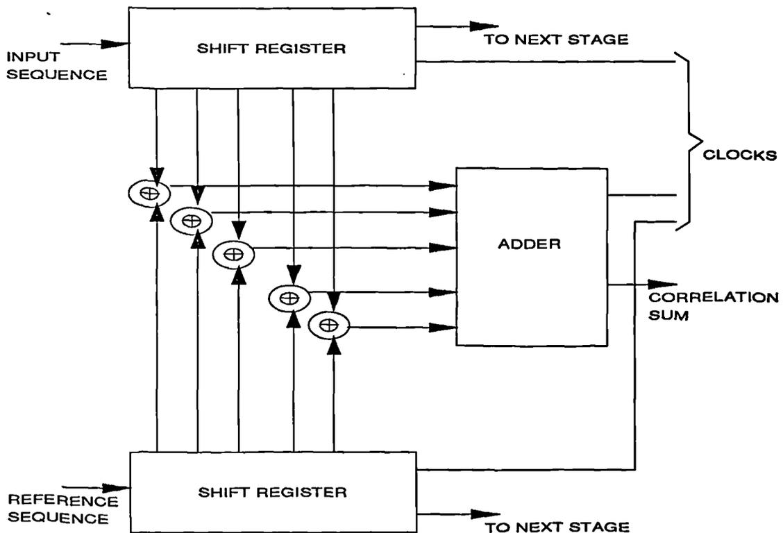
Figure 17 : Block Diagram of Correlator
