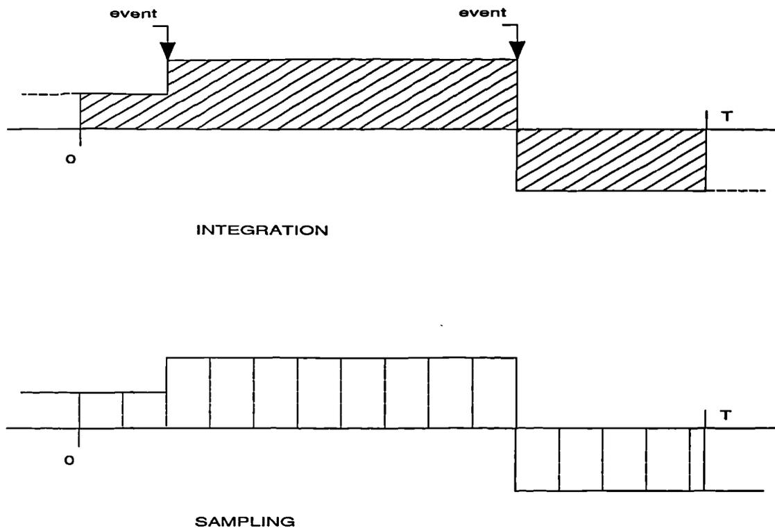
**Figure 13 : Integration and Sampling in the Receiver**
