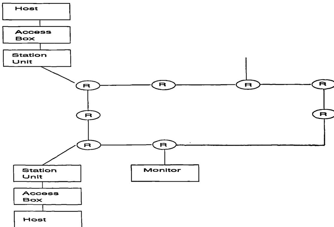
Figure 1 : Slotted Ring Network Topology
