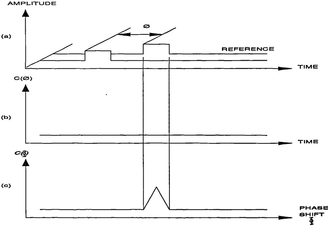
Figure 7 : Autocorrelation Function
