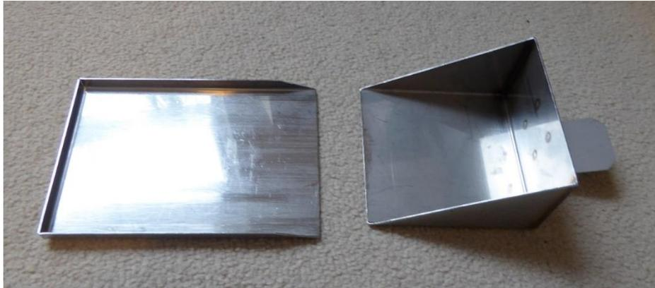
*Figure 3.2. Snowmetrics snow cutter used in this study. This equipment can contain a volume of 250 cm<sup>3</sup> of snow, which together with measuring the snow's weight can be used to obtain snow density.*
