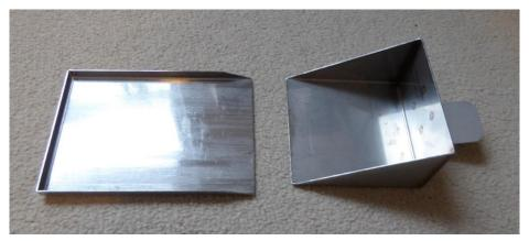
Figure 3.2. Snowmetrics snow cutter used in this study. This equipment can contain a volume of  $250 \text{ cm}^3$  of snow, which together with measuring the snow's weight can be used to obtain snow density.
