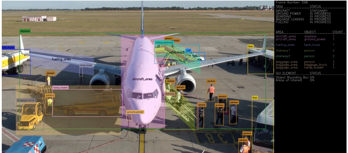
Figure 6.3: Example of an object detection algorithm applied to an image of the aircraft’s turnaround phase. The different kinds of trucks are differentiated and used as a proxy to infer which process is taking place at each time. Image taken from Gorkow (2020) .
