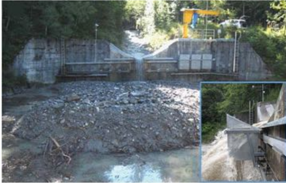
Figure 1.7: The Erlenbach sediment monitoring station, with a zoomed in image of the sediment catching baskets (Rickenmann et al. , 2012).
