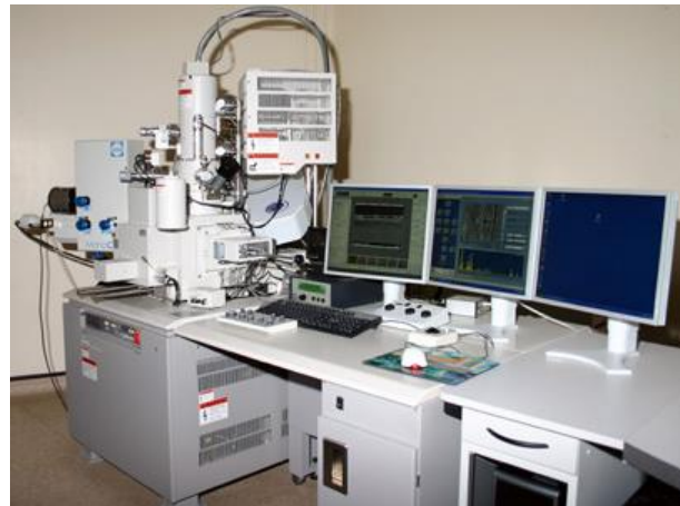
Figure 3.16 Hitachi SU-70 equipment
