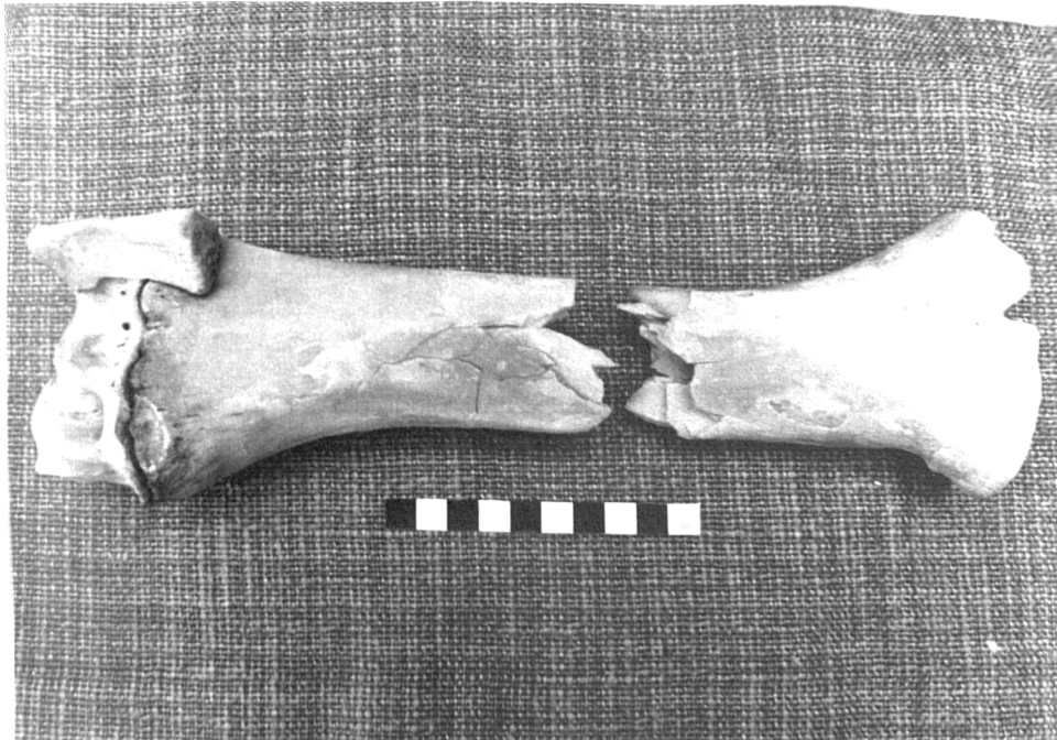
Figure 5.4 - A cow radius fractured after 5 hours in an oven at 80 - 100°C. Features of fresh fracture have been lost.
