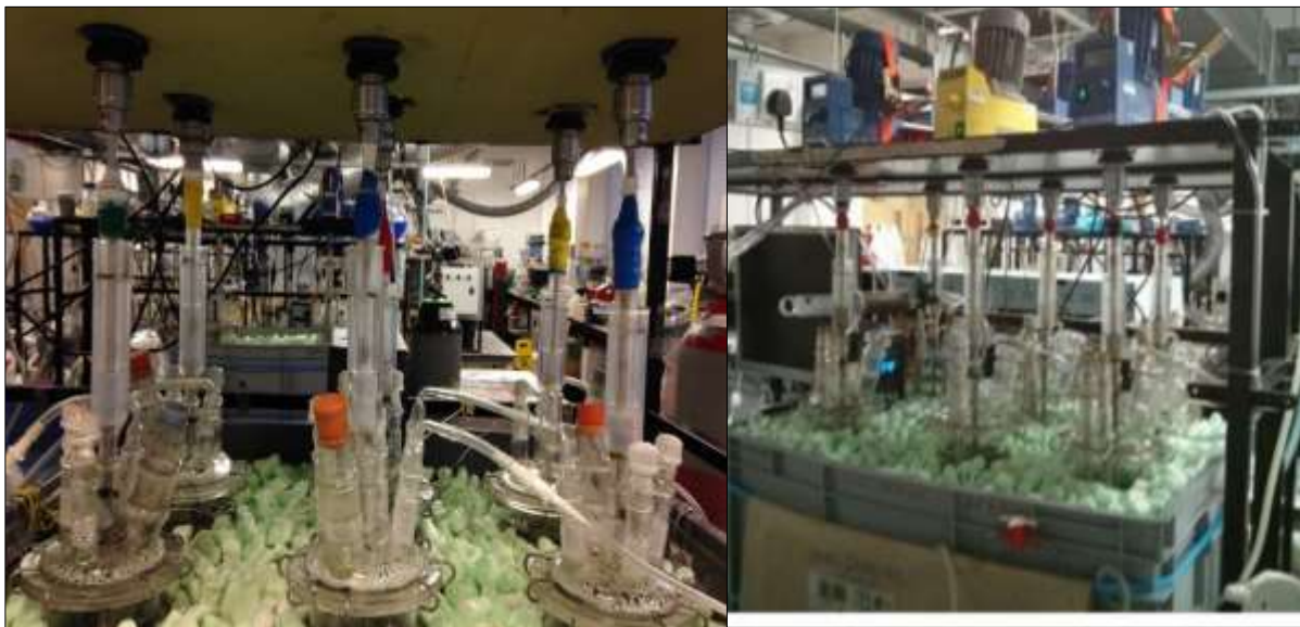
Fig 3-9: A continuous stirred anaerobic bioreactor setting for AD and DF processes (5 L)
