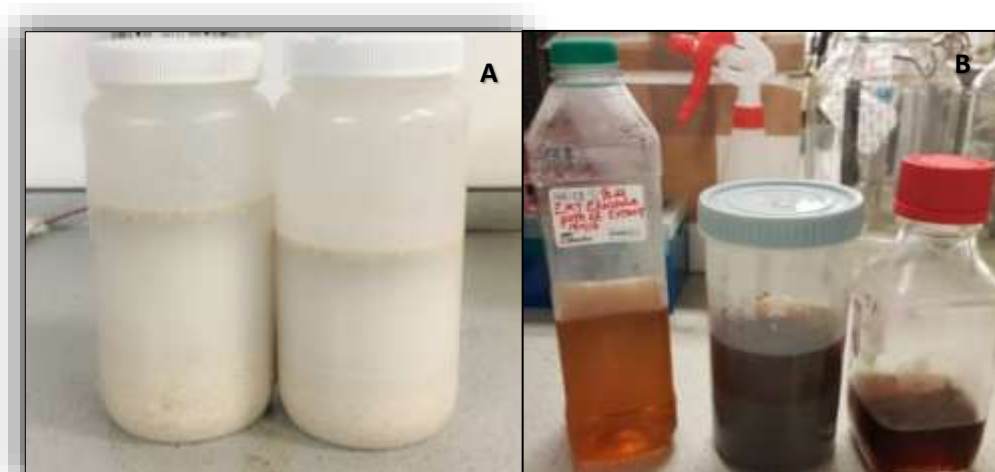
Fig 3-2: A - CSTL extractions (the incubation was done for two days at RT) and B – PE preparation
