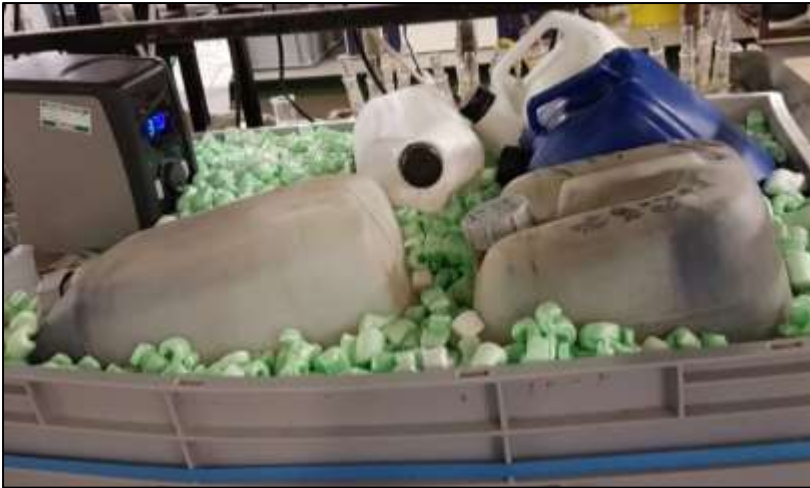
Fig 3-5: Sludge residual incubation (degassing) of seed sludges (ADS and DCS) for 30 days
