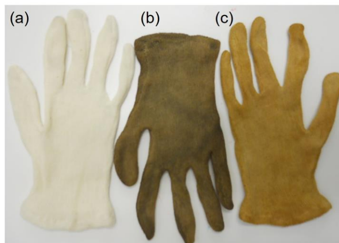
Figure 4.14: Photographs of cotton gloves: (a) uncoated; (b) tea-cinnamaldehyde-silver coated; and (c) tea-cinnamaldehyde-copper coated. 900 mg cinnamaldehyde and 300 mg metal salt added to 300 ml tea solution.
