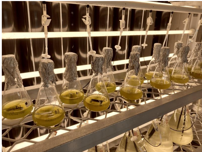
Figure 6.3: Microalgal toxicity apparatus using triplicate 300 ml batch cultures of Chaetoceros calcitrans , Chaetoceros mulleri , and Tisochrysis lutea (T-Iso) in 500 ml Erlenmeyer flasks. Images taken by Mike Packer.
