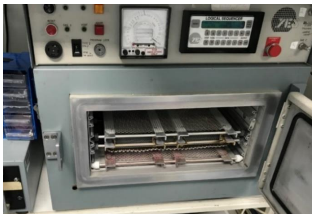
Figure 3.12. UV-oxygen plasma etcher used in this work.
