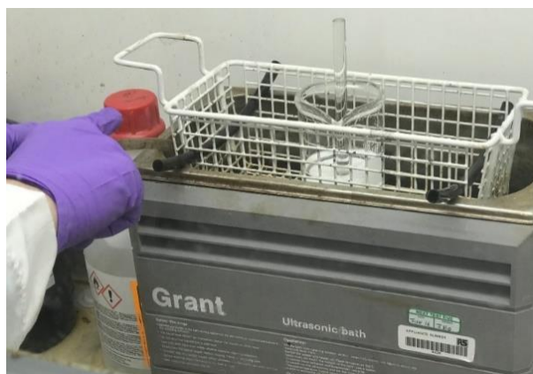
Figure 3.11. Ultrasonic and sonication process used for all device fabrication in this study.
