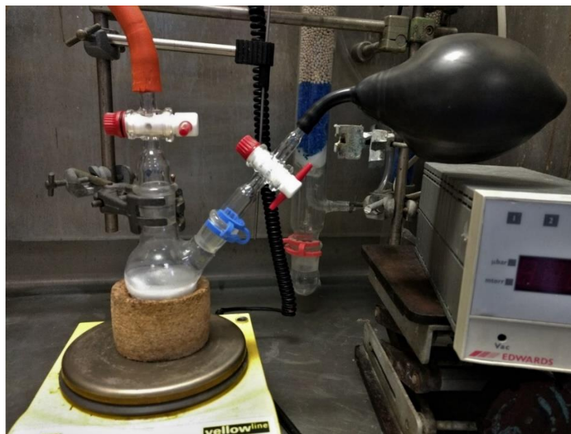
Figure 2.1. Typical gas bladder reaction set-up
