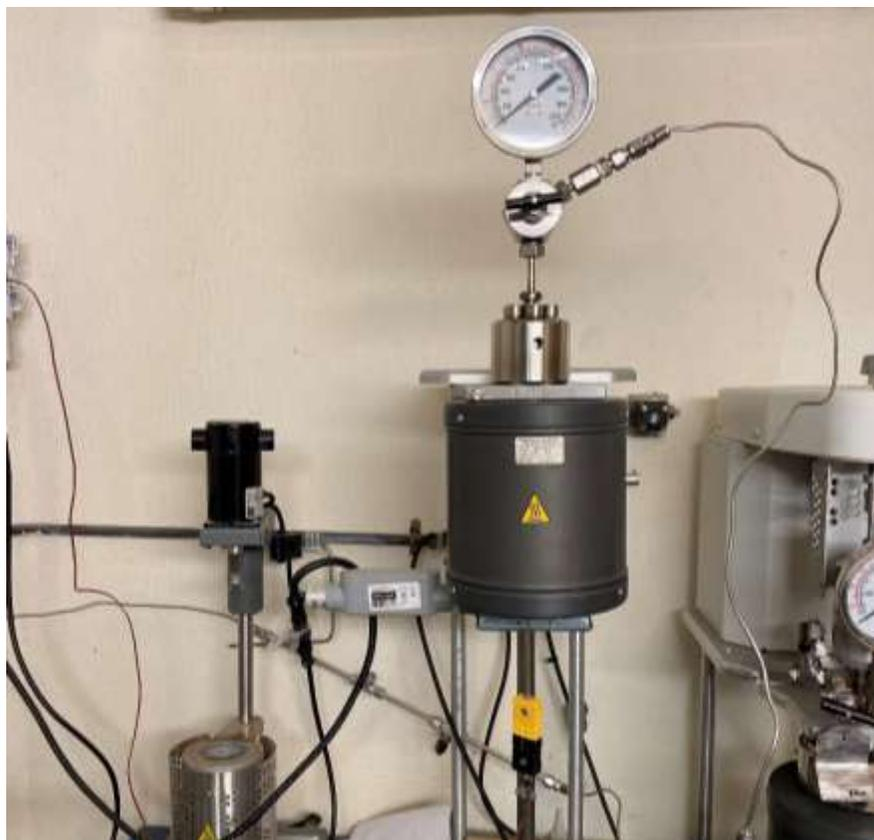
**Figure 2-25.** Parr autoclave set up prior reaction
