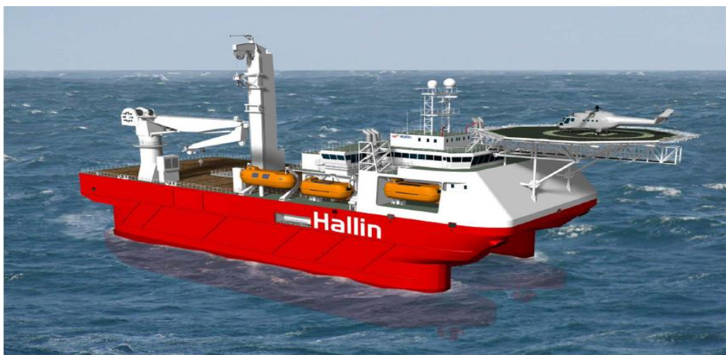
Figure 31: ABS+A1 Mobile Offshore Unit DP3 – Concept vessel [34].
