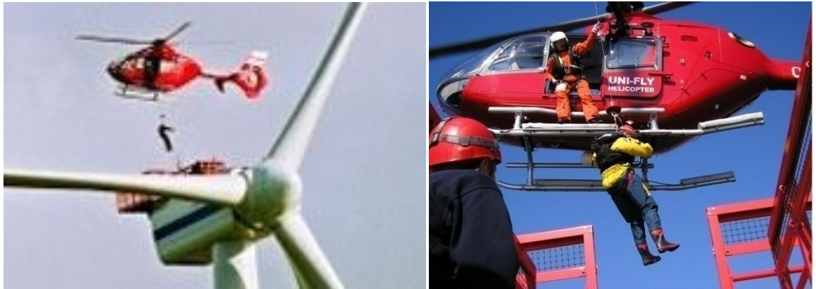
Figure 20: Examples of offshore access to Vestas V80 WT's at Horns Rev by helicopter
