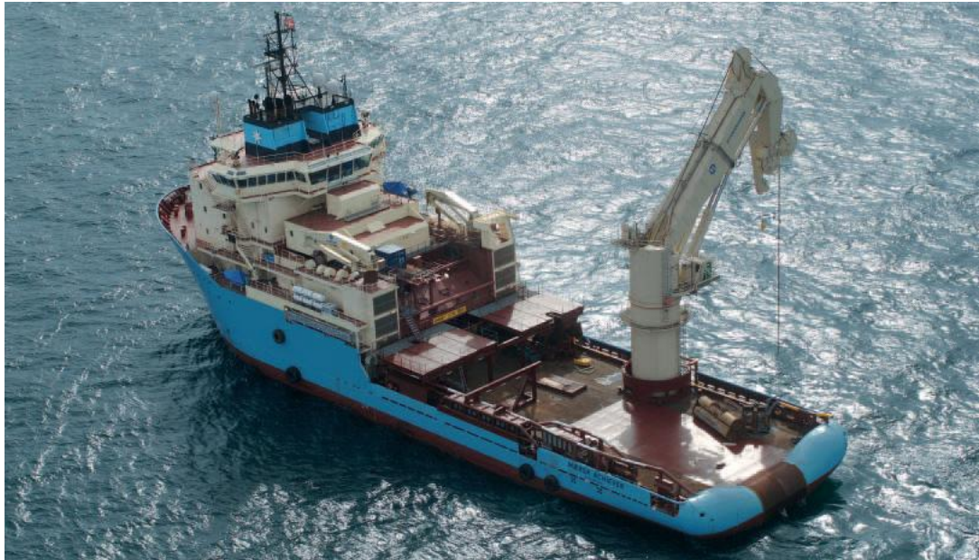
Figure 22: Example of a field support vessel (FSV) [28].
