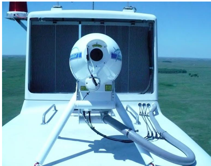
Figure 33: A forward looking laser used to proactively measure wind speed [39].
