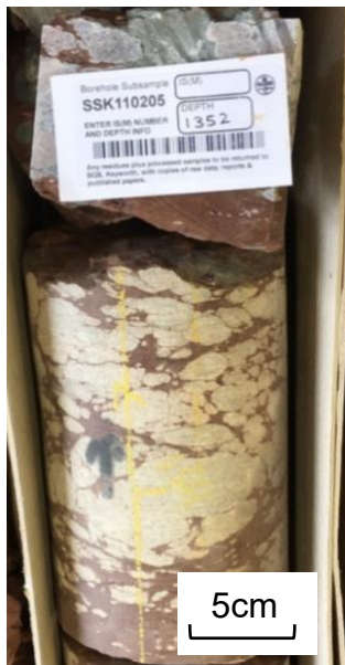
Appendix Figure 10. Large salt nodules, at depth 1,352 ft (412 m).
