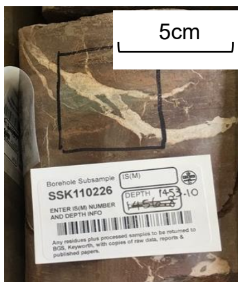
Appendix Figure 13. Anhydrite vein at depth 1,453 ft (443 m).
