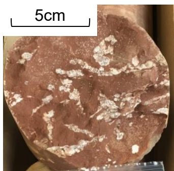
Appendix Figure 2. Micro/macroscale of salt nodules in fine sand mudstone, at depth 3,407 ft (1,038 m).
