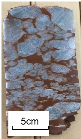
Appendix Figure 9. Large salt nodules cross section (4 cm in diameter) (wet surface), at depth 1,592 ft (485 m).
