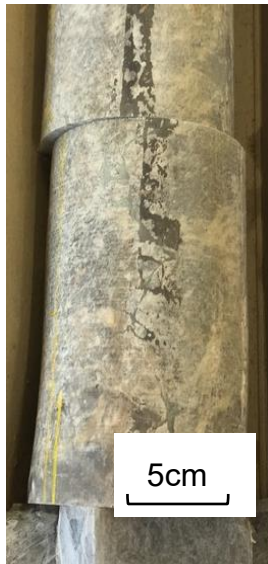
Appendix Figure 12. Anhydrite band at depth 1,334 ft (407 m).
