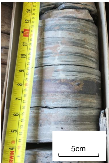
Appendix Figure 6. Grey crystalline anhydrite mudstone, at depth 2,069 ft (631 m).
