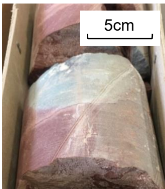
Appendix Figure 4. Green reduction spot (8cm wide), at depth 3,365 ft (1026 m).
