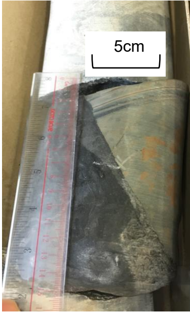
Appendix Figure 6. Grey crystalline anhydrite mudstone, at depth 2,069 ft (631 m).
