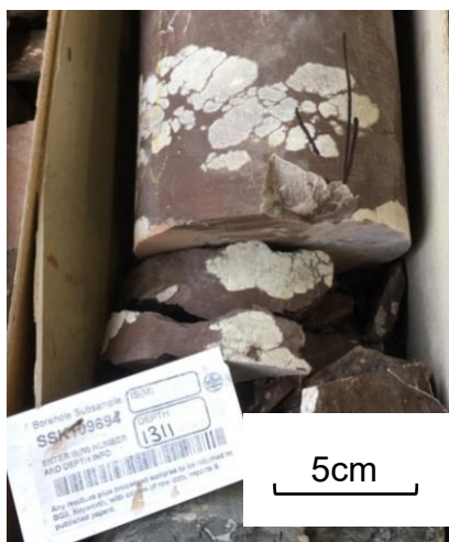
Appendix Figure 11. Salt nodules (~ 2 cm in diameter), at depth 1,311 ft (400 m).
