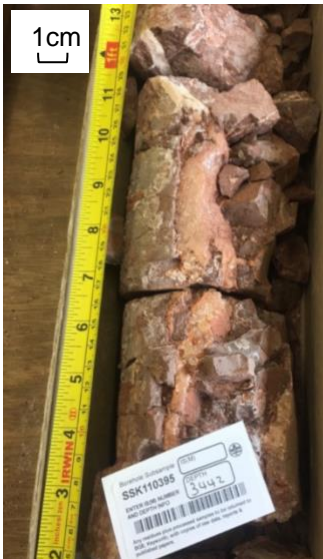
Appendix Figure 1. Vertical salt band (10 inches in length, 3 cm wide) at depth 3,442 ft (1,049 m).
