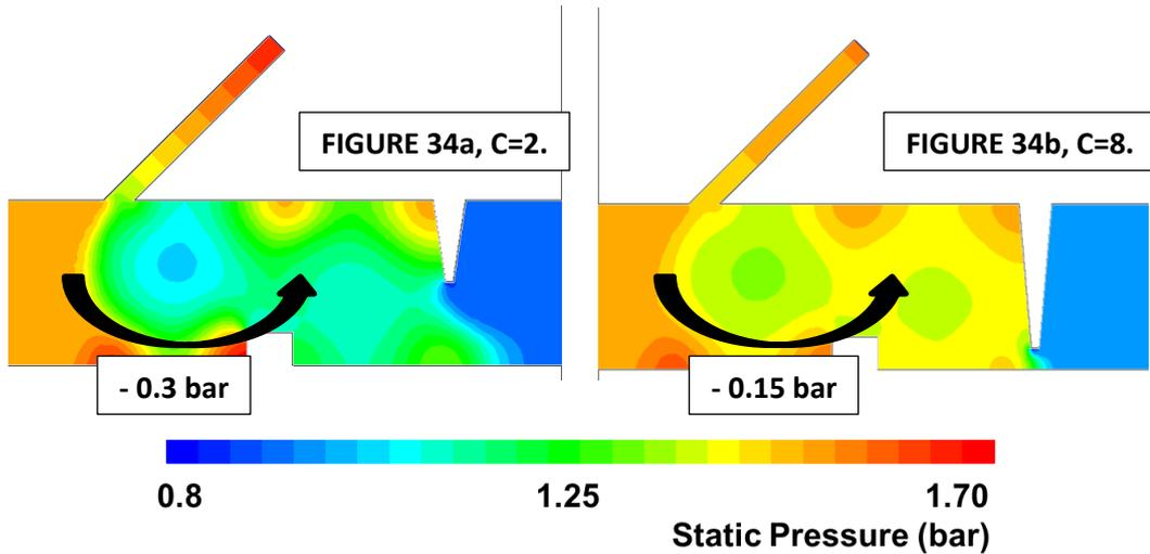
**Figure 34: Static pressure contours for two geometries both with  $A = 8$  &  $D = 2$ . The curtain pressures shown are the closest tested pressure to the overblow pressure for each geometry, Figure 34a shows a  $PR$  of 2.5, Figure 34b shows a  $PR$  of 1.5**
