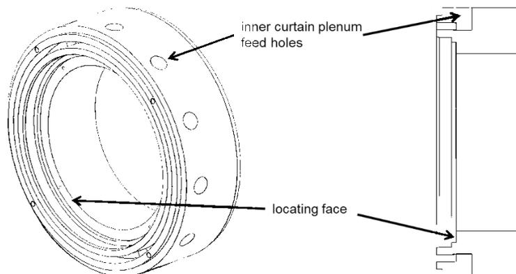
**Figure 45: Curtain plenum rear ring**
