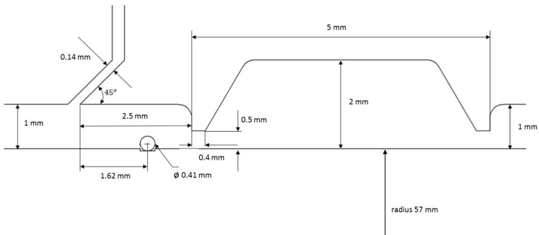
**Figure 40: Hilfer geometry tested using non rotating fluidic seal rig [5]**
