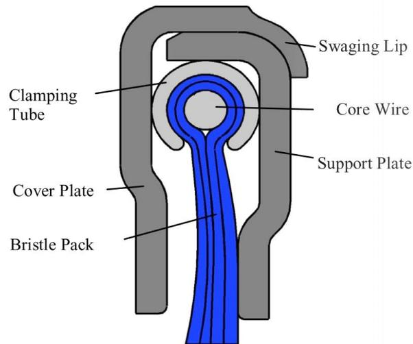
**Figure 15: MTU Brush seal design [23]**
