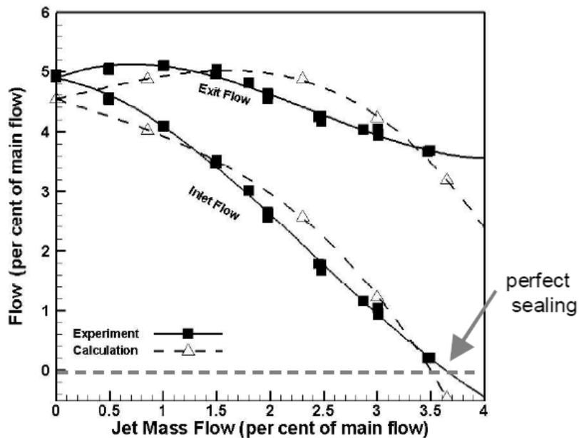
Figure 24: Shroud inlet and outlet flow rates vs fluidic curtain mass flow [9].
