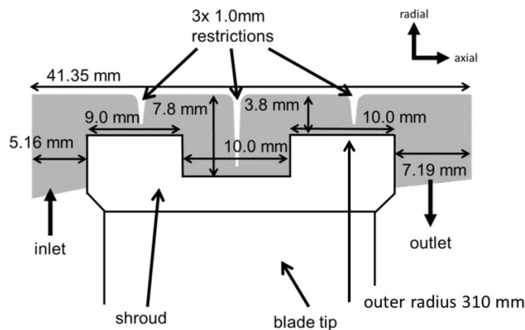
Figure 56: Dimensions of baseline tip seal
