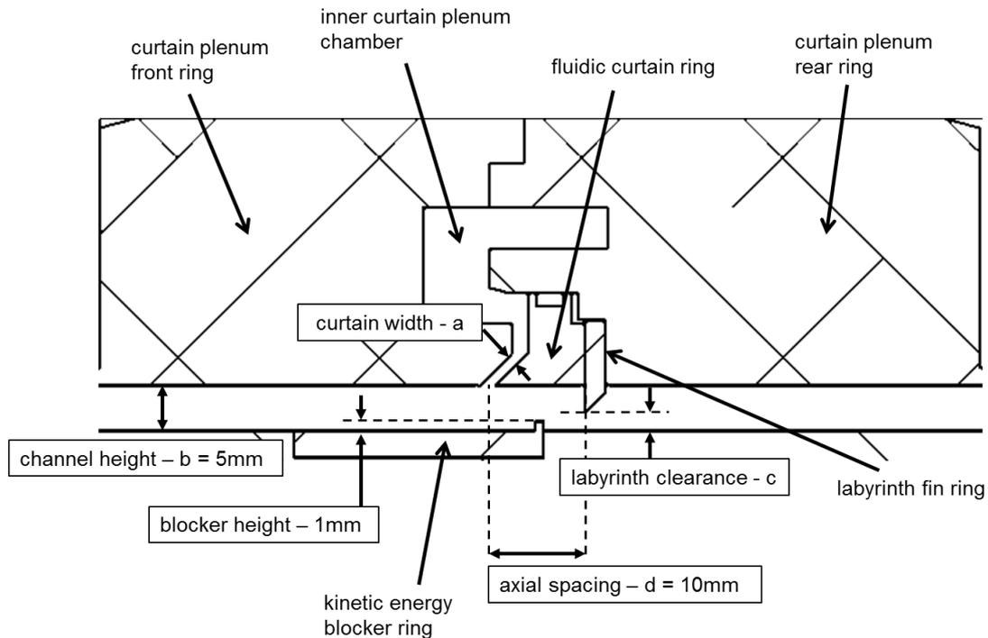
**Figure 43: Section view of modified test rig working section**
