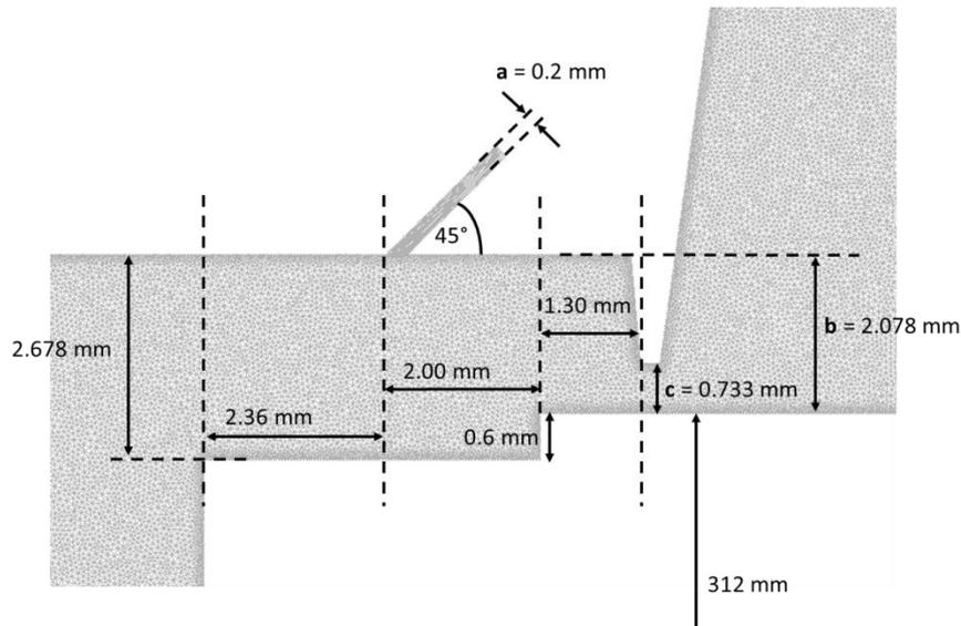
**Figure 71: Dimensions of the Grace seal design.**
