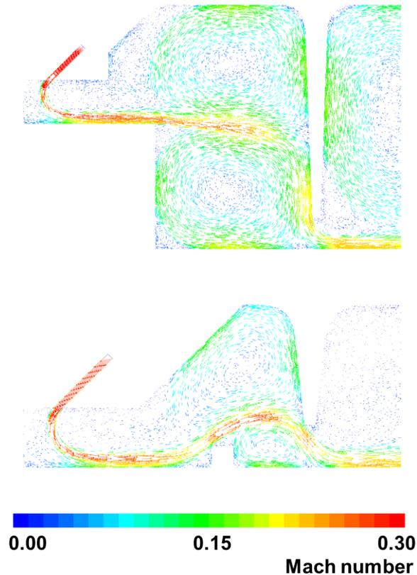
**Figure 65: Velocity vectors where  $A = 8$ ,  $C = 2$ ,  $PR = 1.5$
