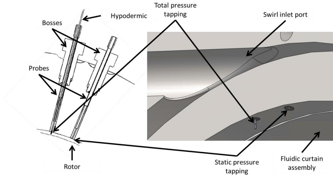
**Figure 92: Section views of swirl chamber pressure measurement ports – left image shows rig-axial view of pressure probes reaching the leakage channel, right image shows a close up oblique view of pressure tapplings**
