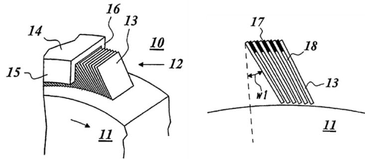
**Figure 16: Sketch of the leaf seal from the original patent [24]**
