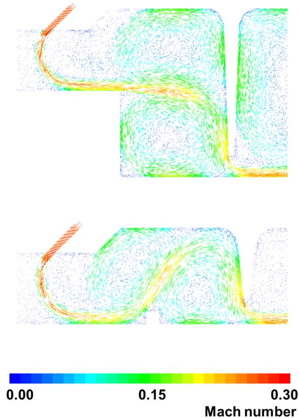
**Figure 66: Velocity vectors where  $A = 10$ ,  $C = 4$ ,  $PR = 1.5$
