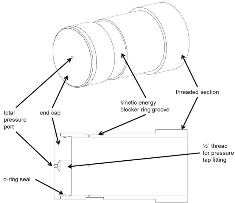
**Figure 48: Inner shaft and end cap**
