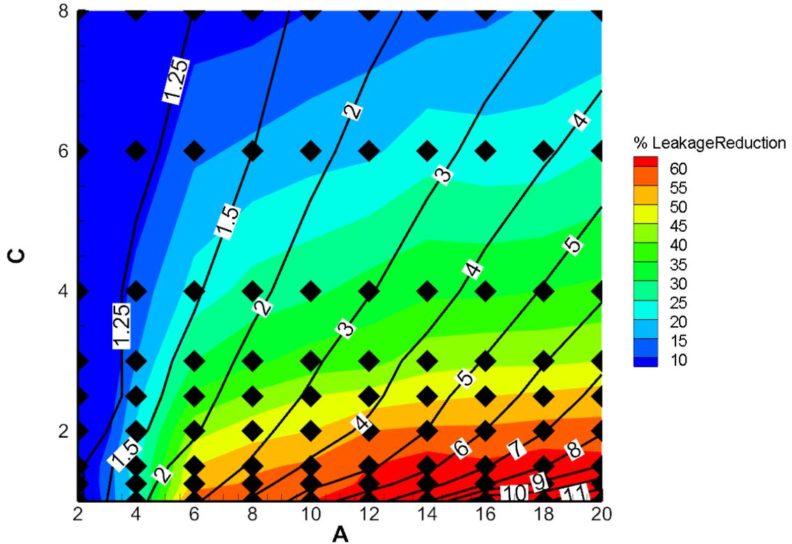
**Figure 33: Max % Leakage Reduction  $L_{max}$  – Generic seal. Bold lines show  $PR_{optimum}$**
