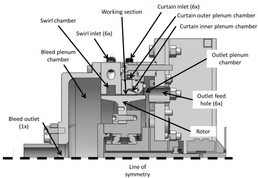
**Figure 87: Section view of the modified test rig**
