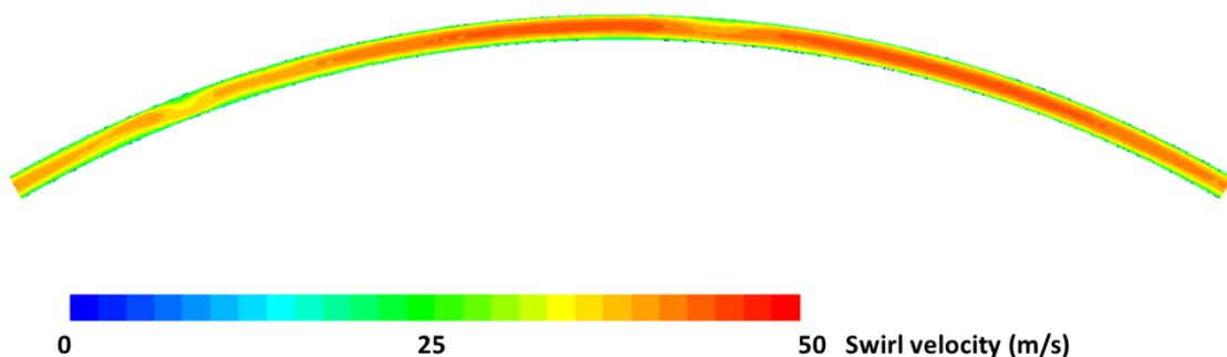
**Figure 91: Contour plot showing the variation in swirl velocity at the position of the fluidic curtain – result corresponds with the second row in Table 21**
