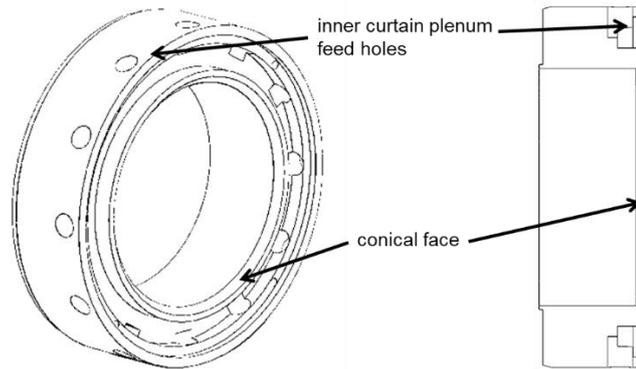
**Figure 44: Curtain plenum front ring**
