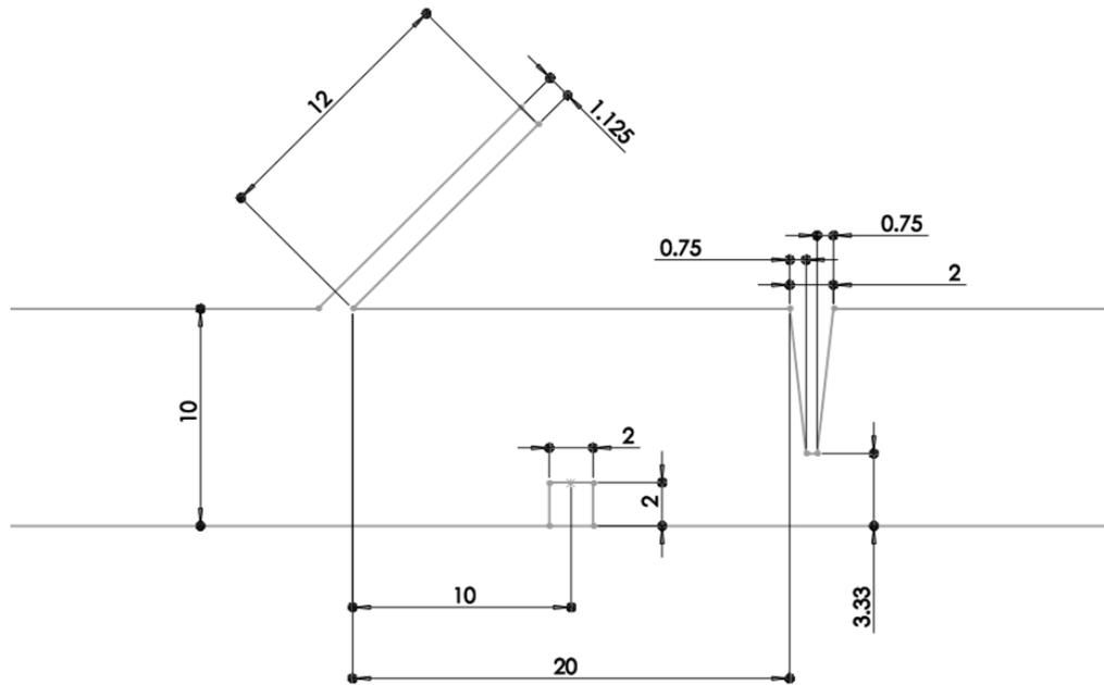
Figure 31: Geometry in case where  $A = 8$ ,  $C = 3$ ,  $D = 2$  (all dimensions in mm)
