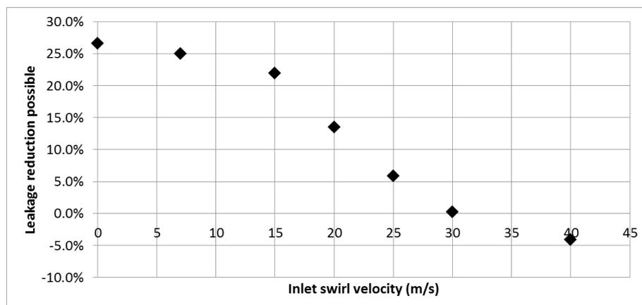
**Figure 78: Maximum leakage reduction vs inlet swirl (R134a)**
