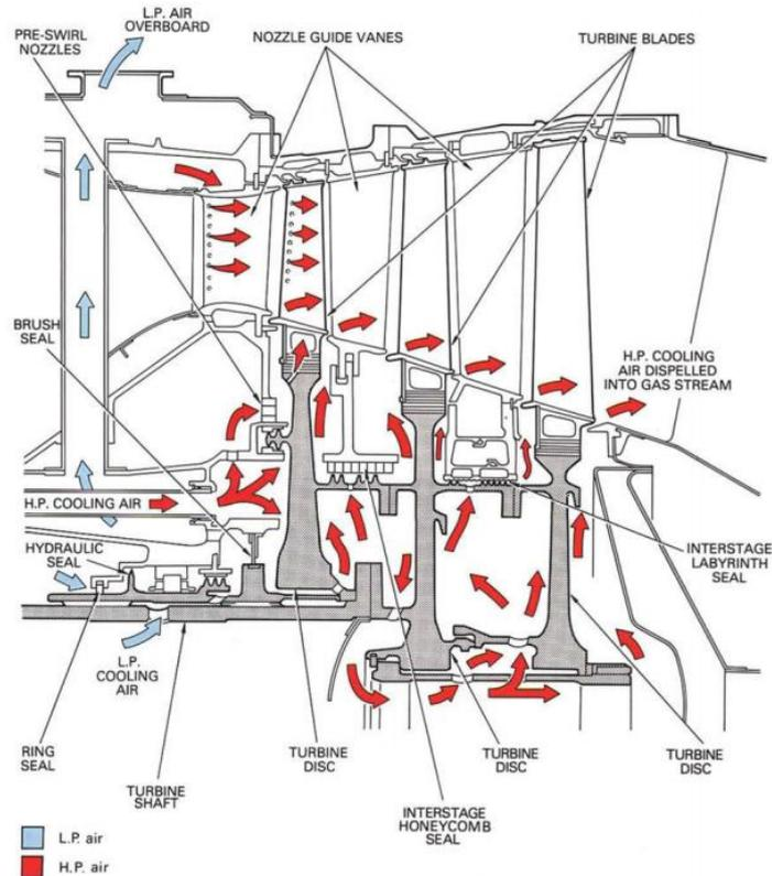
**Figure 2: Example of high pressure turbine secondary air flows.**
