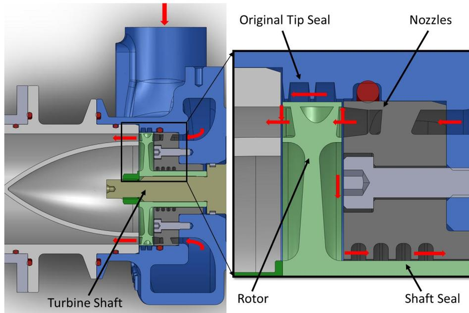
Figure 26: The turbo expander original design [34]
