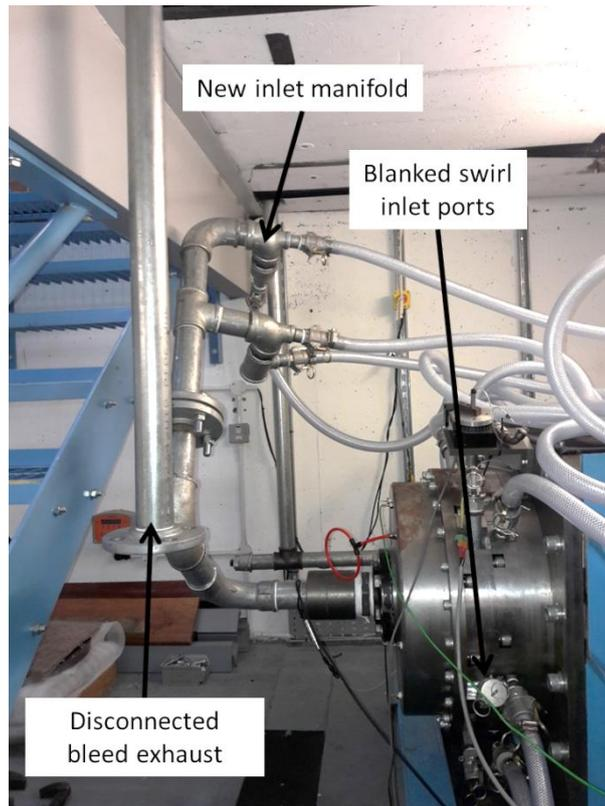
**Figure 96: Test rig in no-swirl configuration**
