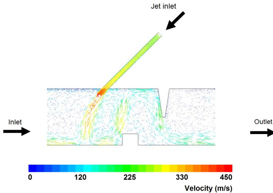
**Figure 36: Velocity vector plot  $A = 12$ ,  $C = 2$ ,  $D = 1$ ,  $PR = 7.0$**
