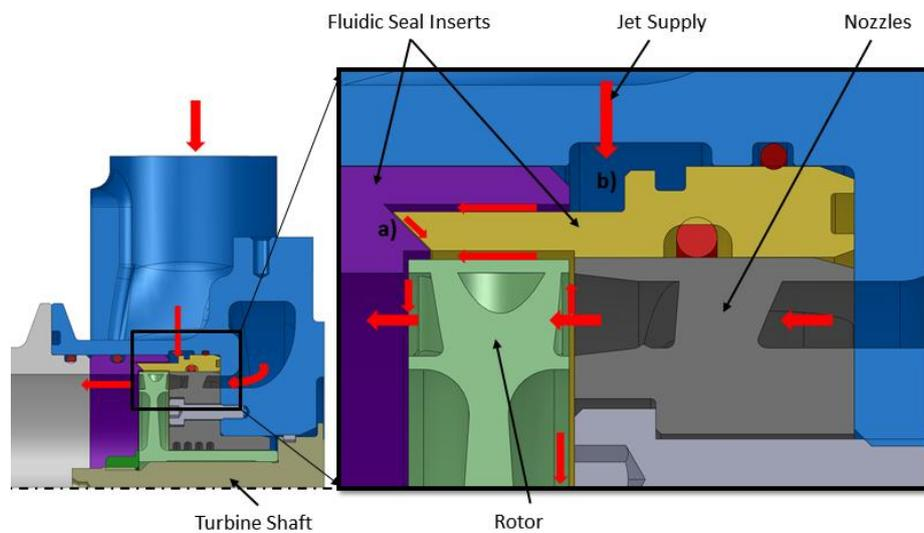
Figure 27: The turbo expander modified design [34]
