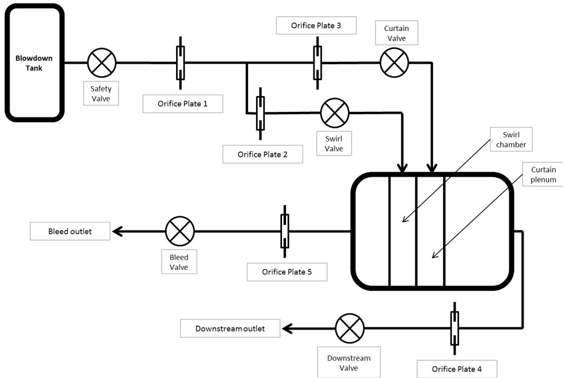
**Figure 86: The rotating seal test rig schematic design**
