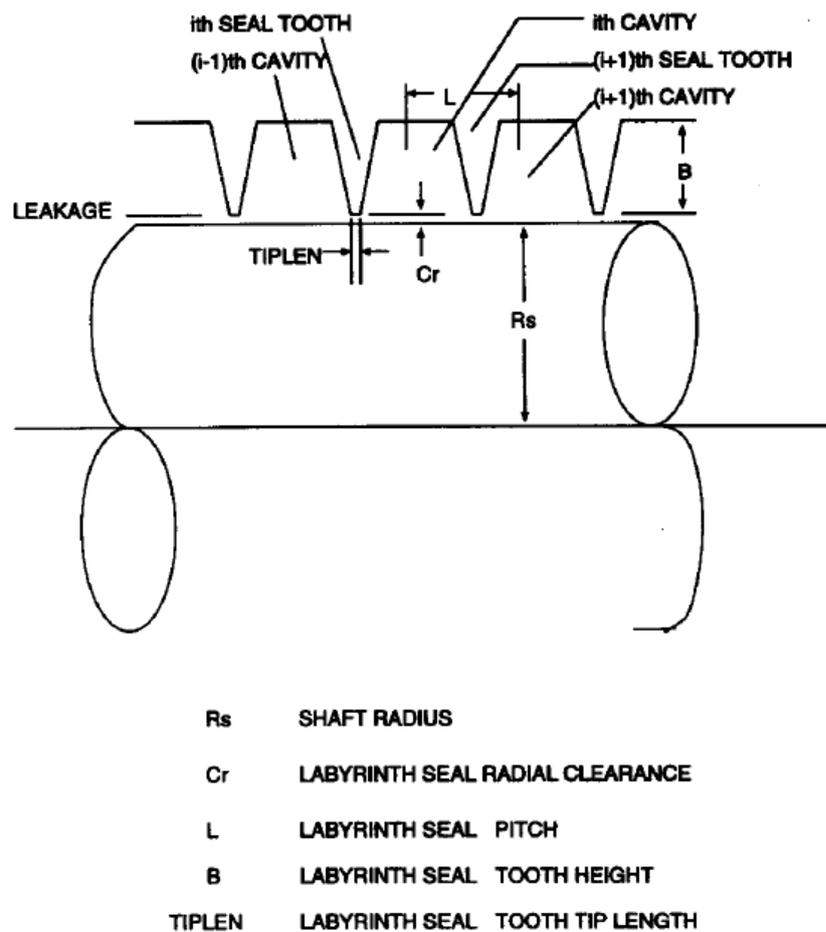
Figure 7: Geometry of a straight through labyrinth seal [14]
