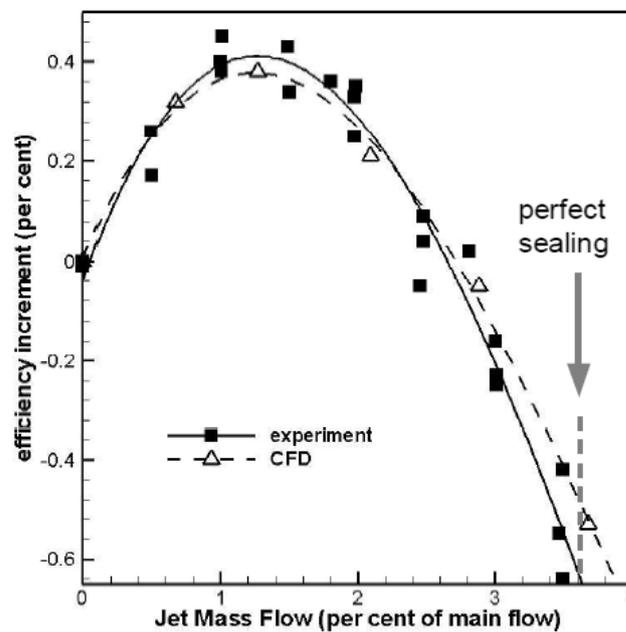
Figure 23: Efficiency change vs fluidic curtain flow [9].
