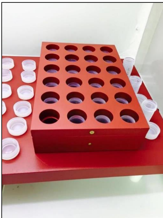
Figure 4.18 Enamel samples in Teflon beakers within on the hot plate following the addition of 8M ultrapure nitric acid.
