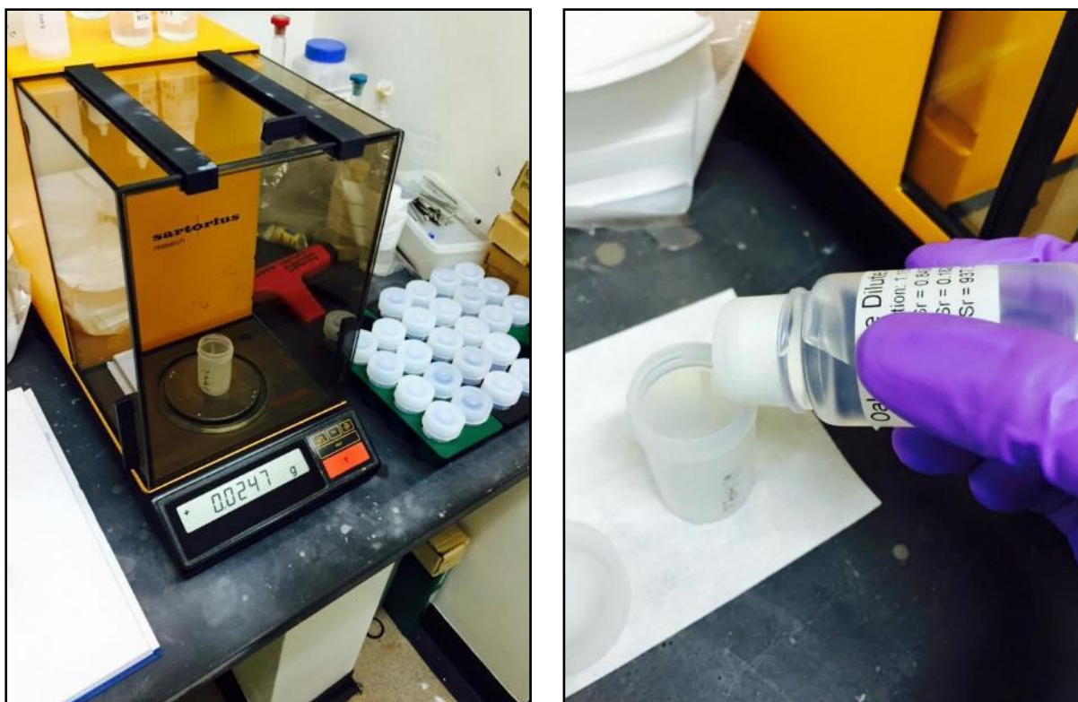
Figures 4.17 Weighing clean enamel samples in Teflon beakers (Left) followed by adding strontium spike solution (Right).
