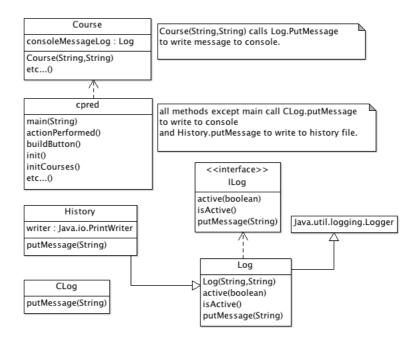
Figure 8.2: Partial CP Class Diagram
