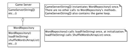
Figure 8.3: Partial PICT Class Diagram
