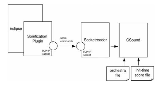
Figure 5.2: System Architecture
