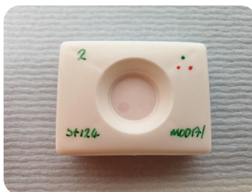
Figure 16 – The flow through chip after the final wash. ST124 shows a spot on the lower left, MOD171 shows an extremely faint spot on the lower right. The top control spot shows no response.
