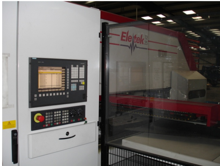
Figure 2.7 - Turret punch machine, microprocessor-controlled fabrication system to be transferred to the CNC machines in the fabrication manufacturing environment
