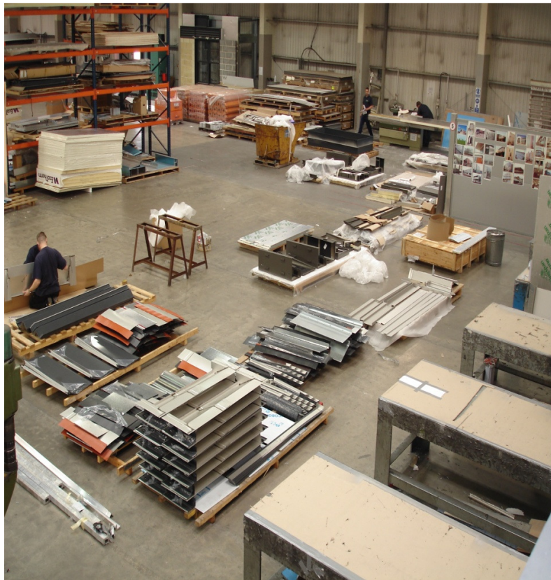
Figure 2.11 - Cladding materials packaged to be shipped to the construction site for installation
