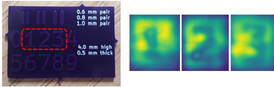
Figure 7.5: Inspection of printed circuit boards (PCBs). Optical ( left ) and THz images ( right ) of copper tracks in a custom PCB. The digits are all 4 mm high with 0.5 mm thick lettering. The copper tracks are visible as darker regions in the THz images when imaged through the surrounding resin board.
