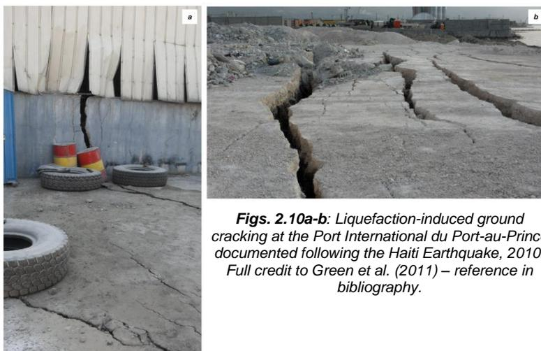
**Figs. 2.10a-b:** Liquefaction-induced ground cracking at the Port International du Port-au-Prince documented following the Haiti Earthquake, 2010. Full credit to Green et al. (2011) – reference in bibliography.
