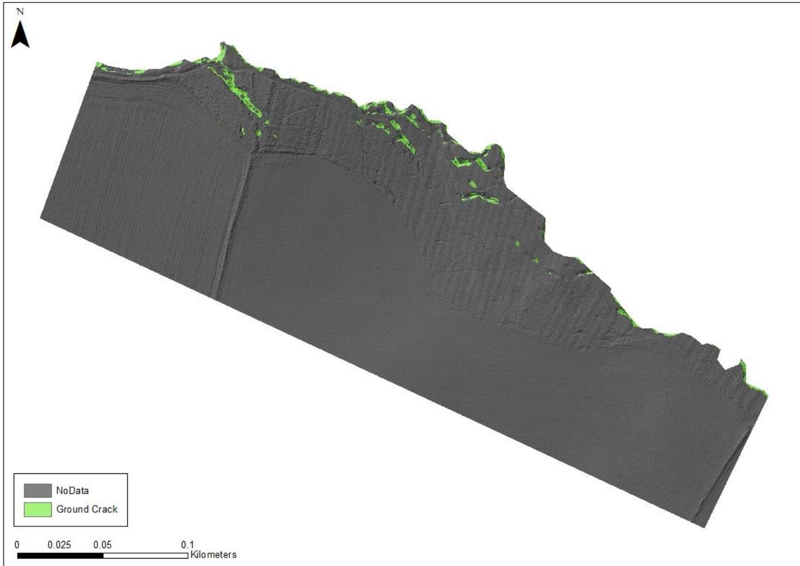
**Fig. 5.07:** Hillshade (0.1 m) overlaid by the final detection attempt using DFME, planform curvature, slope angle and roughness parameters. As can be seen qualitatively, there is a good match between 'ground crack detections' (green) and depressions in the hillshade.
