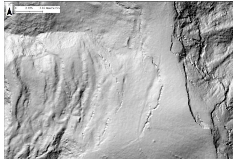
**Fig. 4.02a-c:** Maps showing the visibility of ground cracks from the hillshaded DTM (spatial resolution 1 m). Only the most pronounced features are visible, whilst smaller scale features are much less discernible.
