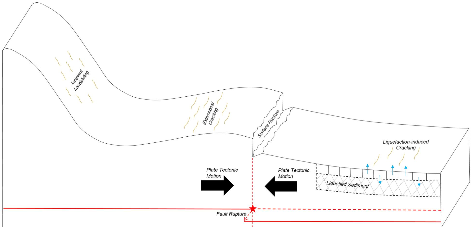
**Fig. 2.04:** An illustration of the different forms of coseismic ground cracking (gold). Coseismic ground cracking can manifest as direct surface rupture, extensional cracking or incipient landsliding as a direct result of strain induced by seismic shaking. Seismic shaking can also cause liquefaction in sediments, which unevenly displaces different parts of the ground (blue arrows), resulting in ground cracking. Adapted from Rajendran et al. (2001).
