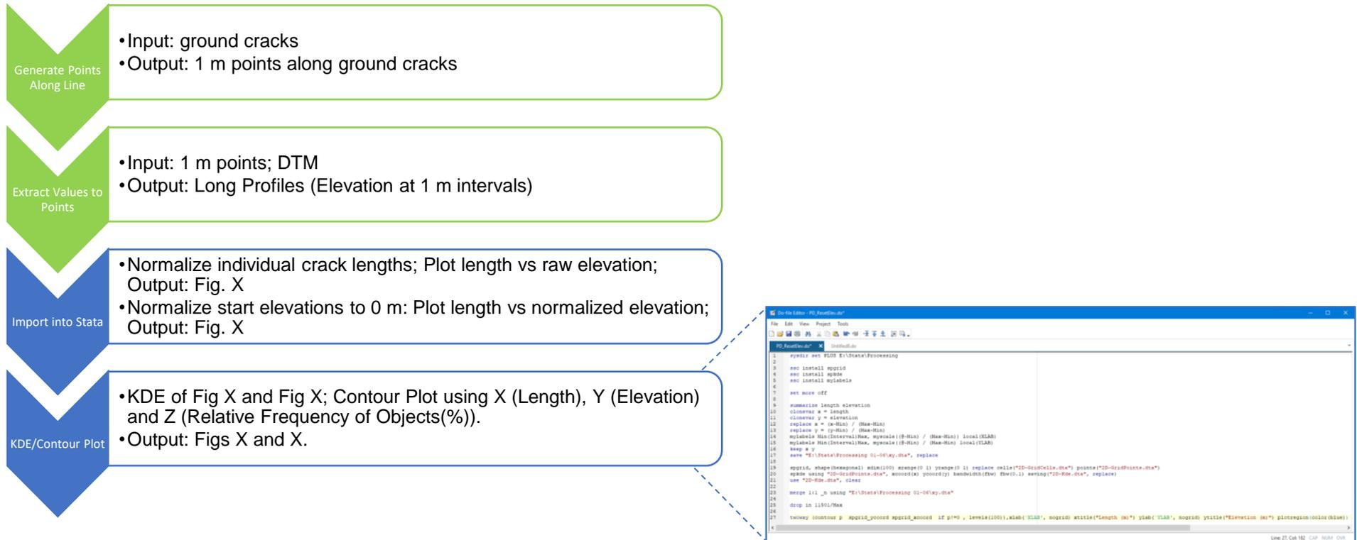
**Fig. 6.04:** Flow diagram illustrating the step-by-step calculation of Long Profile, involving processing in ArcGIS (green) and Stata (blue). The Stata 'Do' file used for the creation of contour plots has been included.
