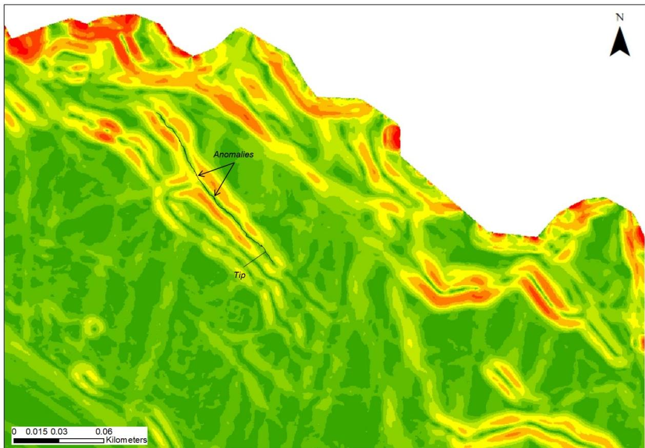
**Fig. 5.04:** Measurement anomalies in crack tips, North Yorkshire, UK. Notice how parts of the same tip (as shown by the arrows) exhibit different slope angle signatures – yellow (top) and green (bottom) respectively.
