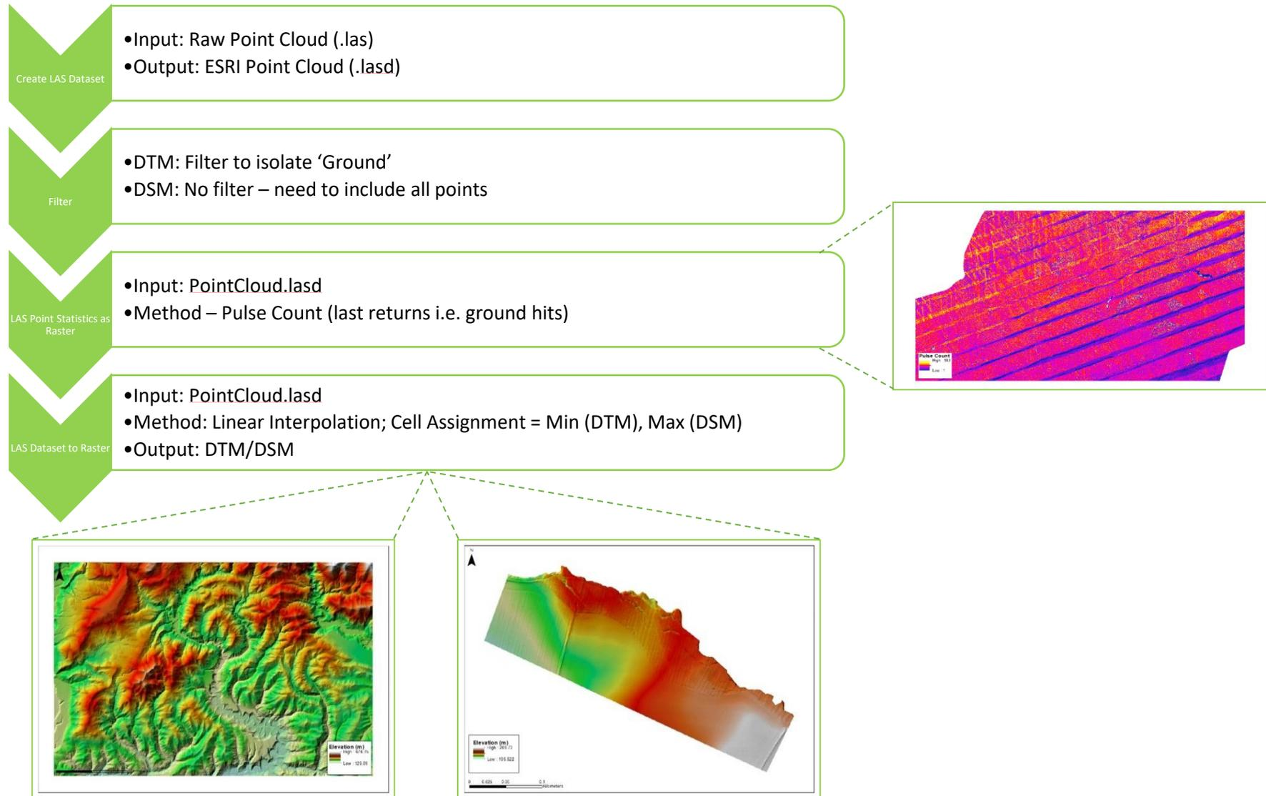
**Fig. 5.01:** Flow diagram outlining the processing of raw point cloud data into an ESRI compatible DTM's for New Zealand (left) and North Yorkshire (right).
