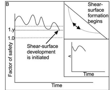
*B: Growth of microcracks results in very small, unnoticeable movements. FoS and v-t space not affected.*
