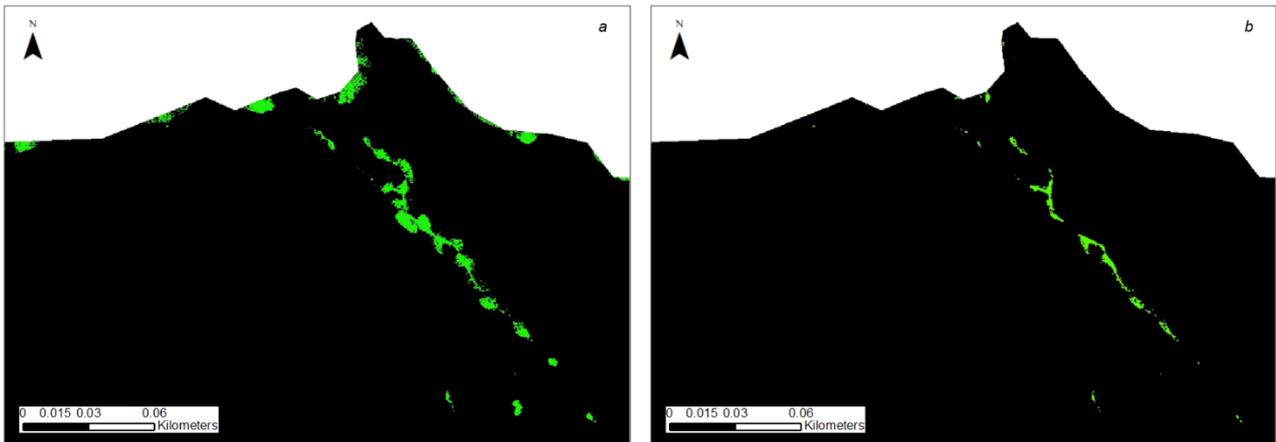
**Fig. 5.05a-b:** Detection attempts before (a) and after (b) the application of SkyView Factor (Kokalj et al., 2011). Notice the reduction in false detections in b compared to a, particularly the green around the cliff edge.
