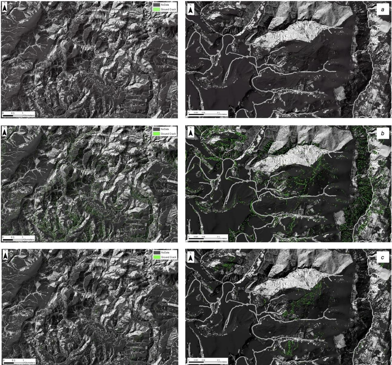
**Figs. 5.09a-c:** Detection attempts using apex signatures (a), wall signatures (b) and a combination of the two (c). Notice the under- and over-prediction in the close-up images of Figs. 5.09a and 5.09b respectively.
