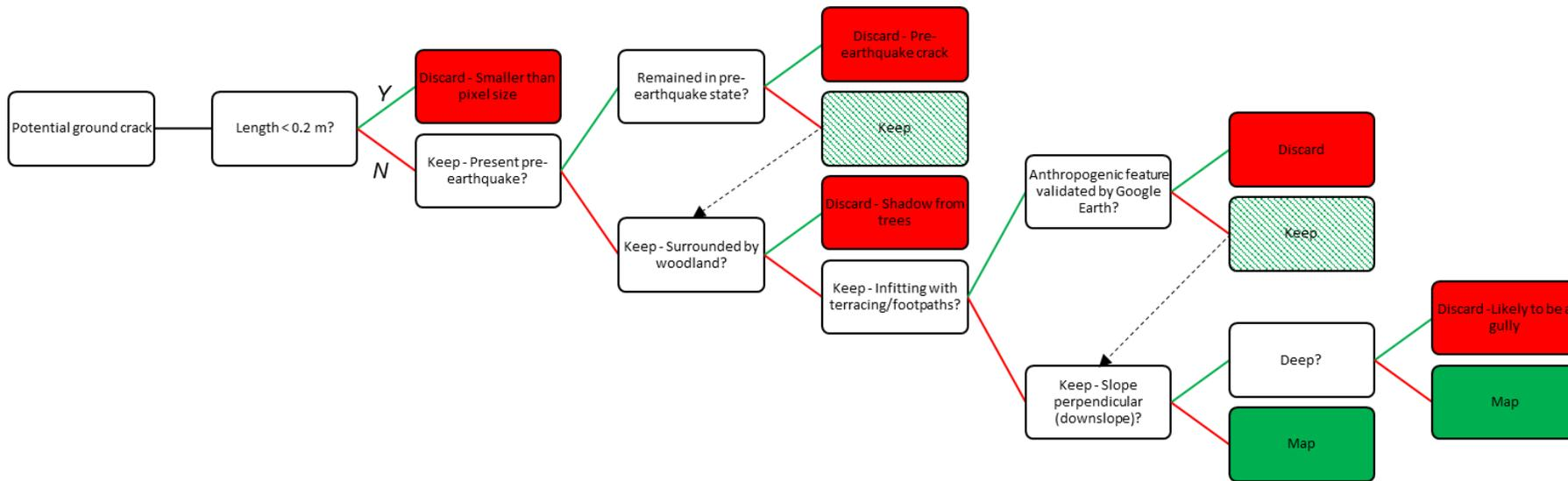
**Fig. 4.07:** Decision tree created for the quality checking of V 1.0 of the ground cracking inventory. This outlines the decision process which was followed when mapping and quality checking each ground crack feature to ensure the accuracy and validity of the final inventory.
