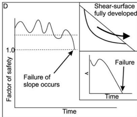
*D: Shear stress exceed shear strength. Linearity takes form in v-t space (e.g. Saito, 1988). Catastrophic failure follows.*
