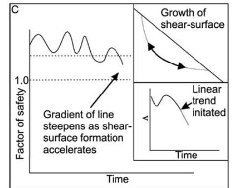
*C: Continued coalescence of microcracks. Results in growth of shear surface. Shear stress on unsheared parts of shear zone increases (eventually hyperbolically (Kilburn & Petley, 2003). Gradients of FoS and v-t space steepen.*
