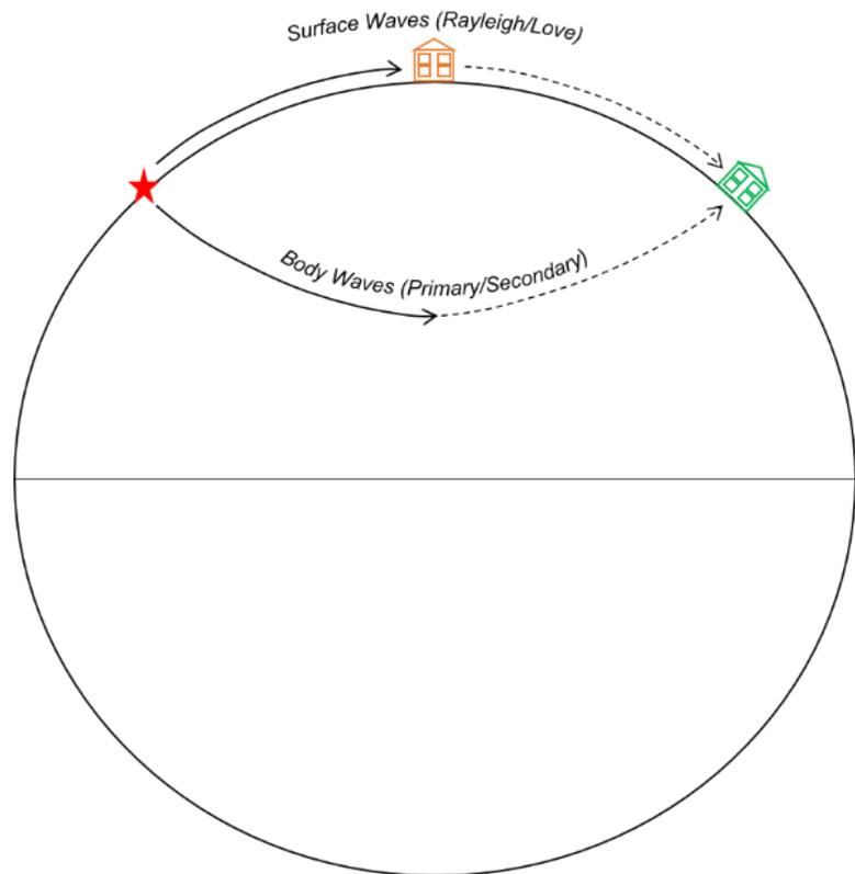
**Fig. 2.03:** A simplistic portrayal of the difference between the propagation of Body Waves and Surface Waves from the Focus. The solid and dashed lines represent the dissipation of energy and consequently shaking intensity. The orange house would therefore experience a higher shaking intensity than the green house. Adapted from Duff (1994).
