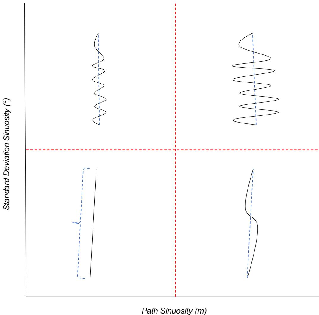
**Fig. 6.11:** Graphical representation of the difference in ground crack form, and how this may be represented through the relationship between path sinuosity and standard deviation sinuosity. Straight lines (blue) are added to aid the visualisation of path sinuosity.
