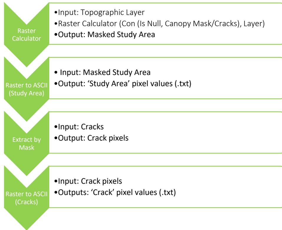
**Fig. 7.02:** Workflow illustrating extraction of study area and ground crack pixels respectively from a topographic/proximal layer. Note that these could be done in tandem.
