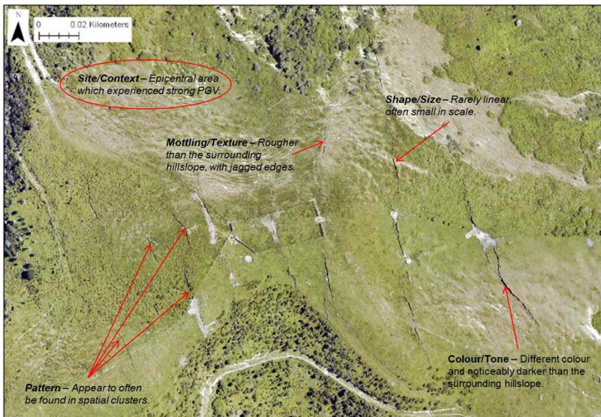
**Fig. 4.03:** An illustration of the characteristics of co-seismic ground cracks which make them discernible for the purposes of manual mapping via visual interpretation. To accompany contextual description in **Table 4.3**.
