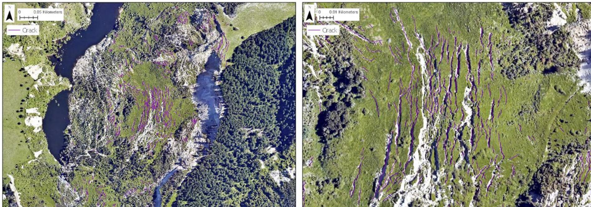
**Fig. 4.04a-b:** **a)** An example of an area of dense ground cracking at a scale of 1:600, which is what was systematically used to initially map ground crack features (purple). **b)** A zoomed in version of Fig.4.04a with a scale of 1:50, showing the dense area of cracking in much more detail. When a dense area of cracking was tackled, zooming in was required to ensure that all features were accurately mapped. Note that this was a source of error.
