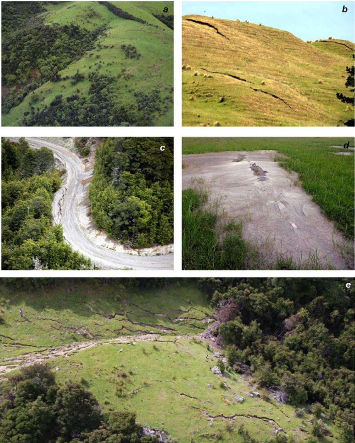
**Fig. 3.12a-e:** Sightings of ground cracking throughout the Kaikoura region documented by Jibson et al. (2018) during immediate post-earthquake field reconnaissance. Full credit to Jibson et al. (2018) – reference in bibliography.
