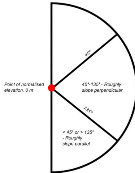
**Fig. 6.03:** Basic diagram to illustrate how long profile shape can be used to indicate the position of ground cracks on a hillslope, through their direction of manifestation from a normalised elevation.
