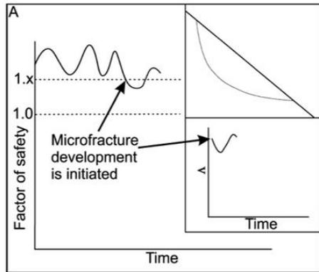
*A: Growth of microcracks results in very small, unnoticeable movements. FoS and v-t space not affected.*
