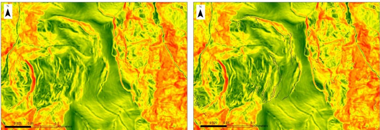
**Fig. 5.08a-b:** Unlike the North Yorkshire dataset, the New Zealand dataset is not precise enough to be able to distinguish between ground crack apexes and walls. **a)** This is the slope layer applied to the New Zealand dataset, where ground cracks only show one signature as opposed to two in the North Yorkshire dataset for crack walls and tips respectively. **b)** Same as **Fig. 5.08a**, but with the addition of ground crack polygons for context.
