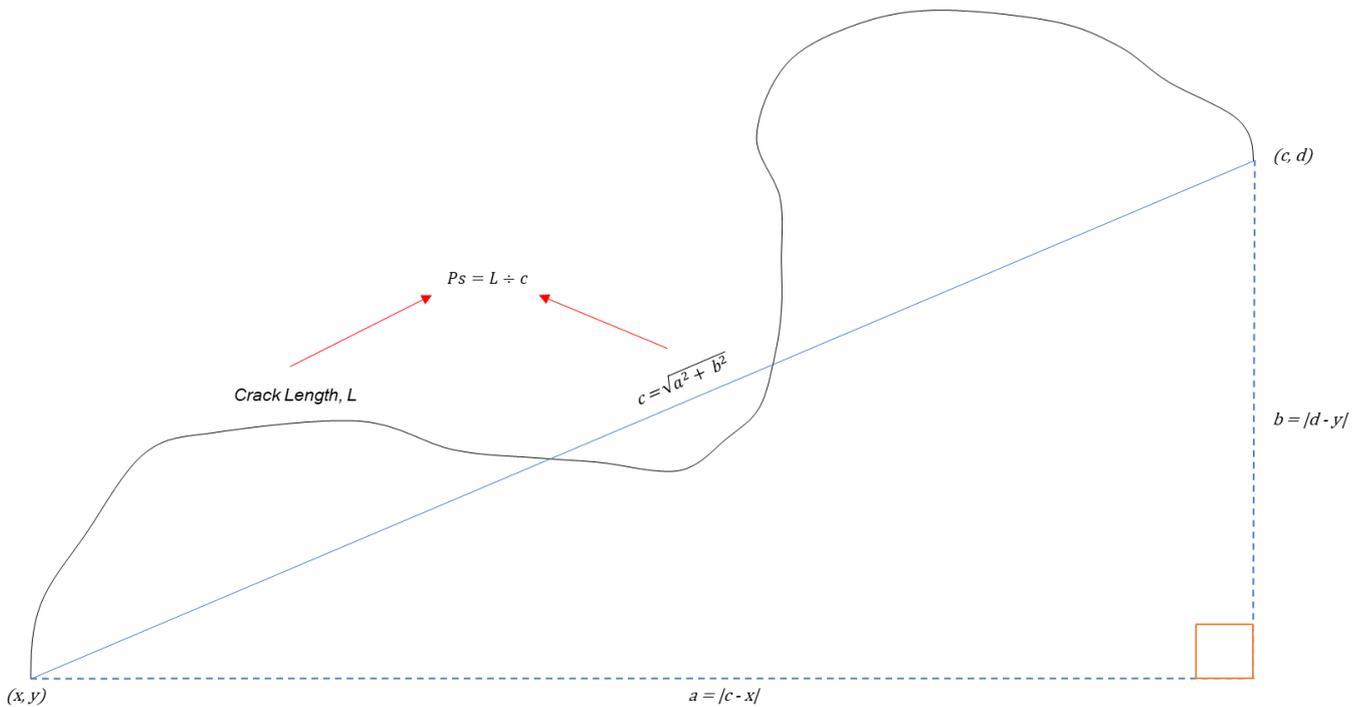
**Fig. 6.12:** Diagram of path sinuosity ( $P_s$ ), showing the difference between crack length (black) and straight line length (blue) and how the latter is calculated using start/end coordinates, and then Pythagoras' Theorem. Crack Length,  $L$ , is supplied in the polygon Attribute Table.
