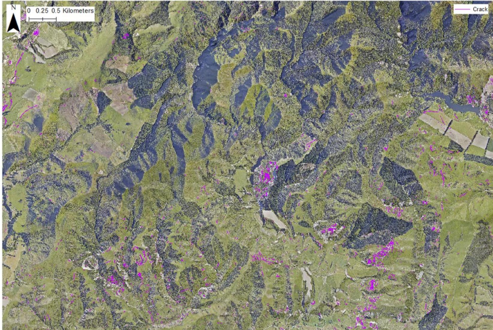
**Fig. 4.08:** A map illustrating the final, quality checked, ground crack inventory produced from manual mapping via the visual interpretation of aerial imagery.
