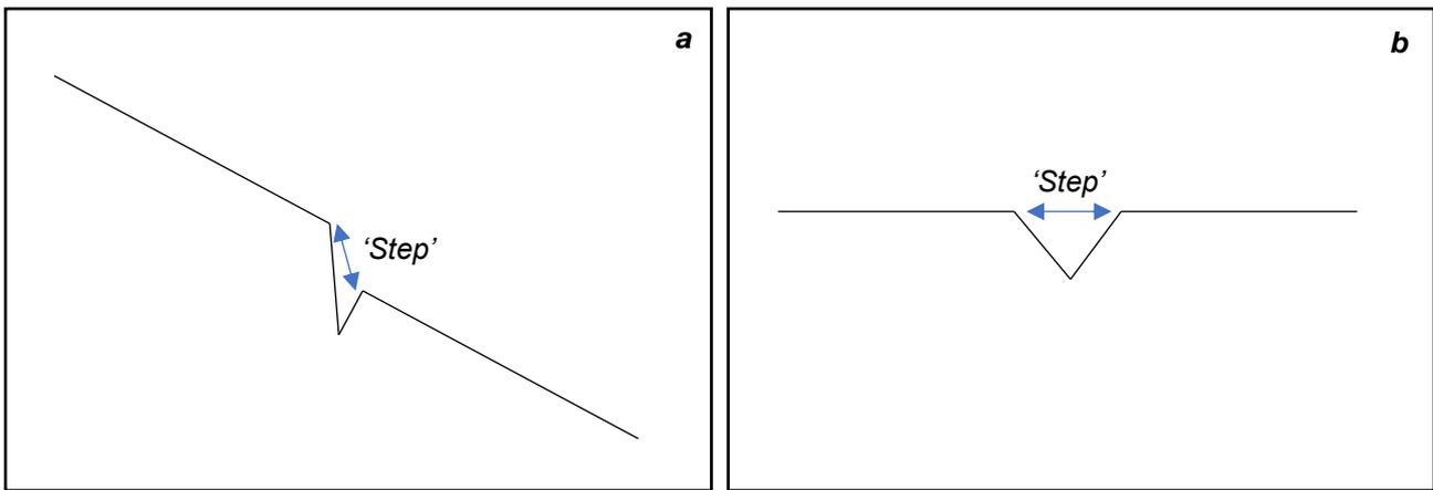
**Figs. 6.05a-b:** Diagram depicting how the extension mechanism of ground cracks may differ depending on whether they occur on: a) A hillslope, where steeper gradients may result in more of a 'step-like' extension mechanism, or b) Flat ground, where the gradient may lead to a 'cleaner' extension.
