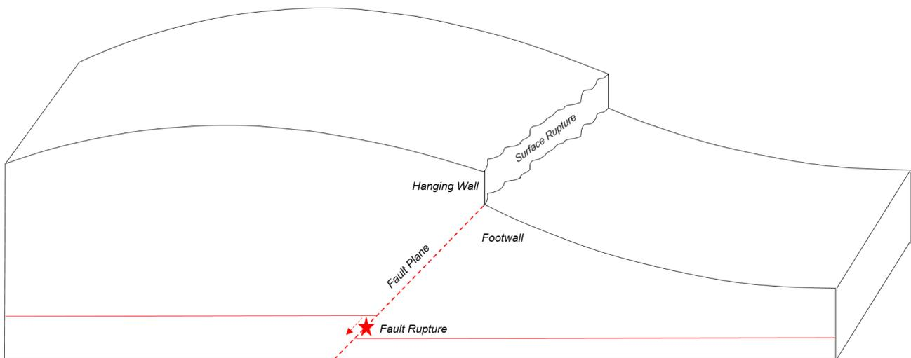
**Fig. 2.02:** An illustration of the hanging wall and the footwall, showing their position in relation to the fault plane.
