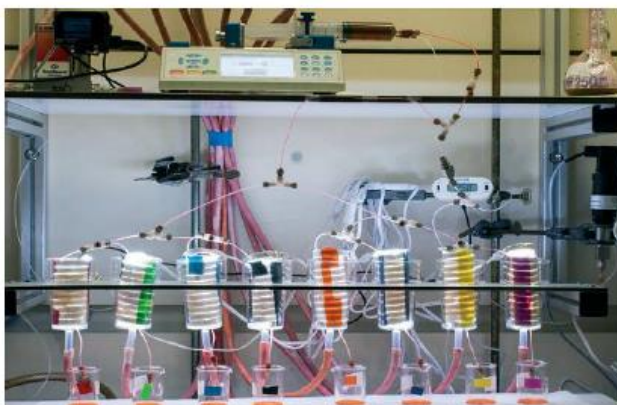
Figure 9: An example of numbering up for reaction scale up.
