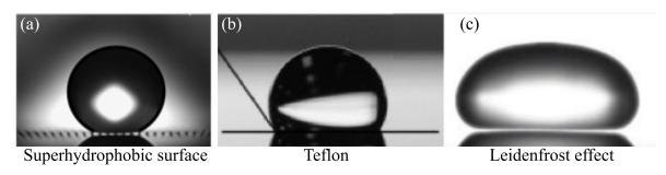
Figure 1.8: Droplet shapes on liquid repellent surfaces observed using a goniometer: (a) A droplet on superhydrophobic surface. The air pockets underneath the droplet are visible [41]. (b) A droplet on a hydrophobic surface obtained from Teflon coating which demonstrates a relatively high contact angle [42]. (c) Levitating droplet on a metallic surface exhibiting the Leidenfrost effect [43].
