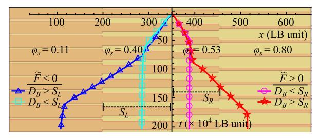
Figure 5.11: Potential applications of LIS with topographical gradient. With multi sections of stepwise gradients, droplets can be classified from their sizes, represented by their base diameter  $D_B$ , by controlling the sections' width, here  $S_L$  and  $S_R$ .
