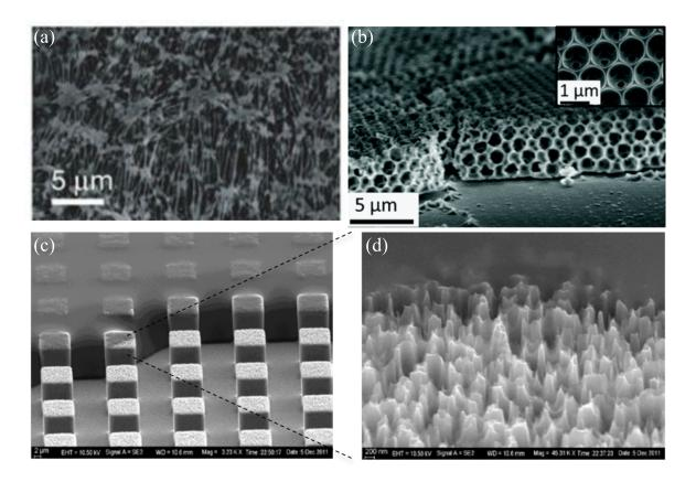
Figure 1.12: Examples of surface textures for LIS: (a) commercially available Teflon microfibre membrane [58], (b) inverse opal [64], and (c) mircoposts with (d) secondary roughness in form of nanograss [57].
