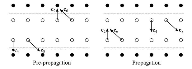
Figure 2.4: Illustration of how the no-slip boundary condition is achieved by implementing the bounce back rule such that if  $f_i$  is propagated in the direction of  $c_i$ , it will be reflected back in the direction of  $-c_i$ .
