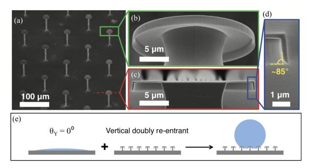
Figure 1.9: (a-d) Scanning electron micrographs of a textured surface with reentrant geometries. (e) The reentrant geometry significantly increases the energy barrier which prevent the droplet to collapse into the surface porosity, event for a complete wetting fluid [48].
