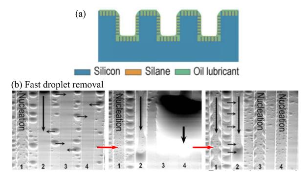
Figure 7.3: Application of LIS as a fog harvesting surface [127]. (a) Schematic of the grooves type LIS with multiscale surface texturing design. It reveals that the lower scale rougness is imbibed with oil lubricant, while the higher scale roughness remains unfilled. (b) The fabricated LIS demonstrates fast droplet removal.
