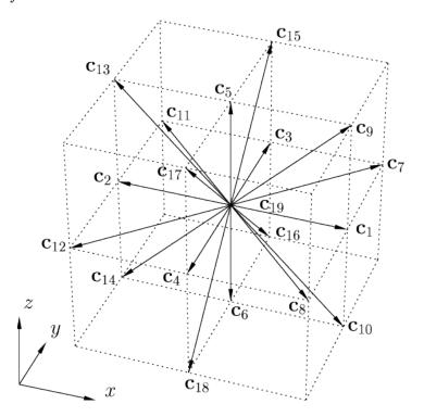
Figure 2.1: A unit cell of D3Q19 lattice velocity model. The  $\boldsymbol{c}$ 's represent the discretised velocity directions.
