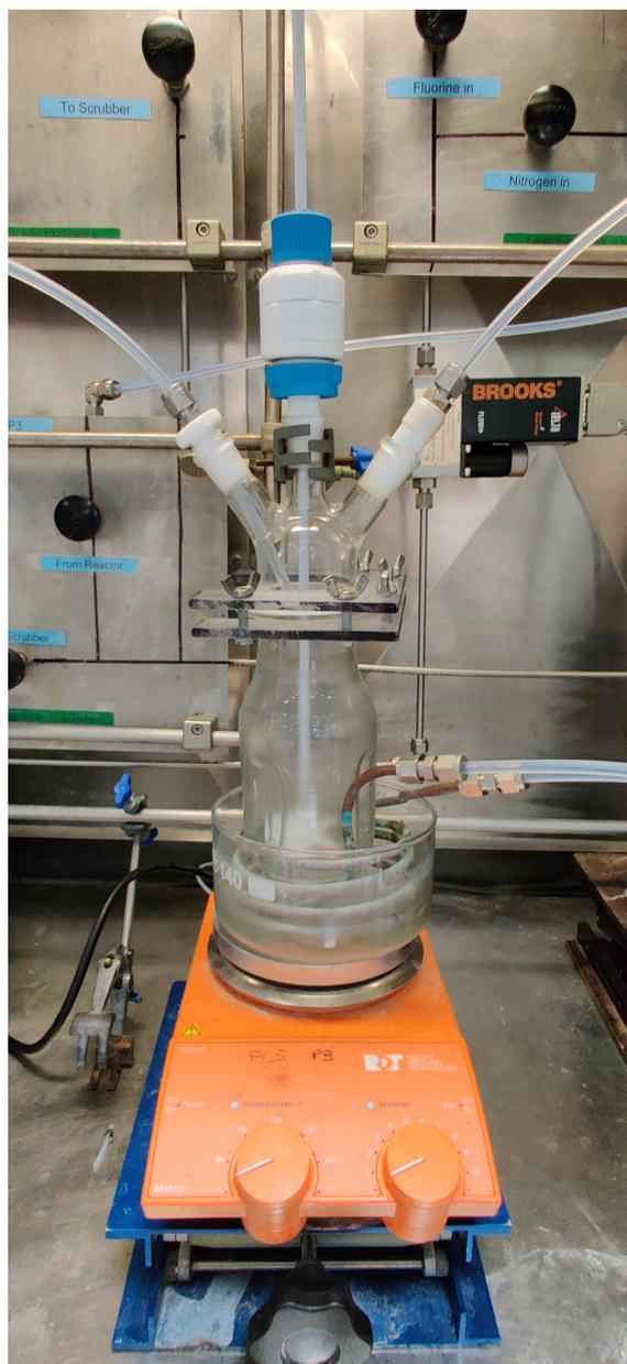
Figure 8.2: Large scale ( $\leq 20$  mmol) fluorination set-up
