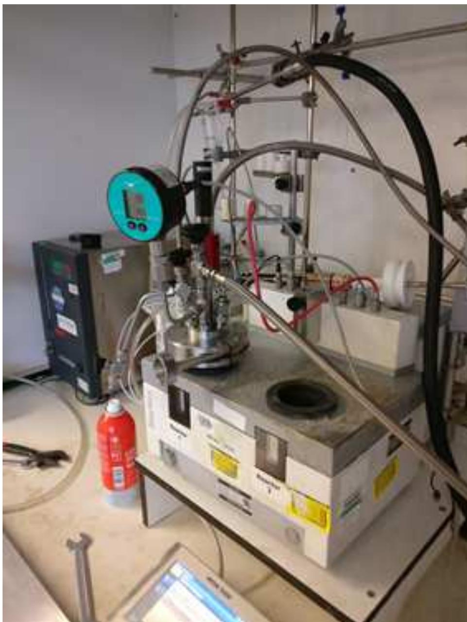
Figure 4.16: Hydrogenation of 1-(difluoromethyl)-4-nitrobenzene using an EasyMax reactor
